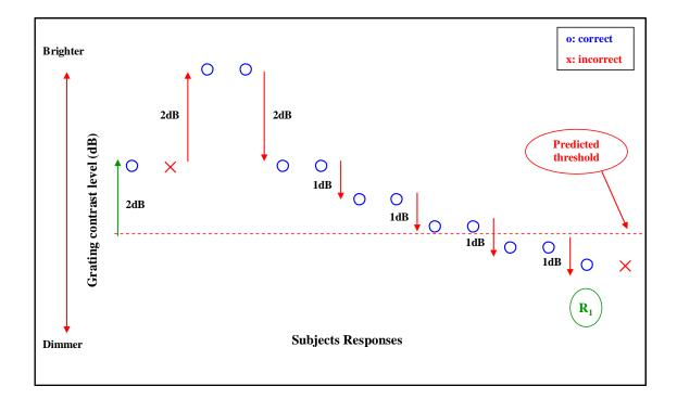
Figure 7.19 A schematic of the staircase algorithm for any one of the 41 non-seed points, where one reversal determines the length of the staircase.
