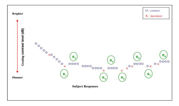
**Figure 7.1** A schematic of the 'Proof of Concept algorithm' where 8 reversals determines the length of the staircase, and the geometric mean of the last 6 reversals is used to calculate the final threshold.  $R_1$  through to  $R_8$  represents the corresponding reversal.
