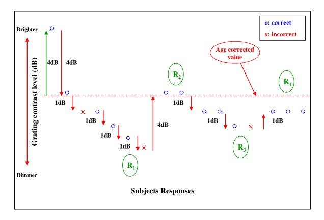
Figure 7.4 A schematic of the staircase algorithm where 4 reversals determine the length of the staircase, and the final reversal is used to calculate threshold. The final threshold is 1.50dB below the age-corrected value.  $R_1$  through to  $R_4$  represents the corresponding reversal.
