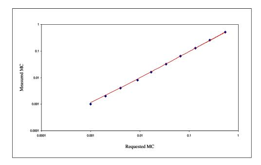
**Figure 4.3** The  $log_{10}$  of the measured Michelson contrast against the  $log_{10}$  of the requested Michelson contrast following gamma correction.
