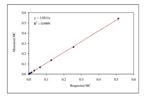
**Figure 4.4** The untransformed measured Michelson contrast against the untransformed requested Michelson contrast following gamma correction. The linear fit is constrained to pass through the origin.
