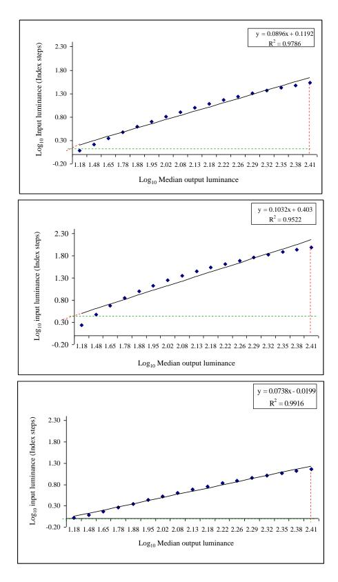
**Figure 4.1** The Log<sub>10</sub> of the input luminance, expressed in index steps, against the Log<sub>10</sub> of the median output luminance for the red (top), green (middle) and blue (bottom) colour guns. The y intercept and the slope of the function, together with the Coefficient of Determination,  $R^2$ , are given in the top right of each panel.
