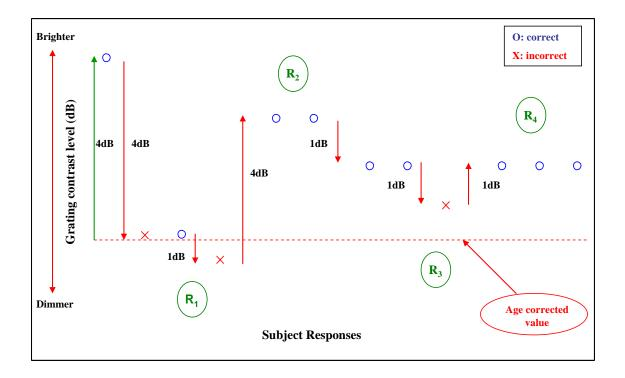
Figure 7.3 A schematic of the staircase algorithm where 4 reversals determine the length of the staircase, and the final reversal is used to calculate threshold. The final threshold is 1.5dB above the age-corrected value.  $R_1$  through to  $R_4$  represents the corresponding reversal.
