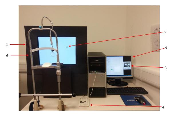
**Figure 2.4** The prototype Dynamic Noise Perimeter. 1, the monitor displaying the stimulus. 2, the stimulus without the noise mask. 3, fixation monitoring. 4, the keyboard for recording a response. 5, the monitor displaying the operating menus. 6, the adjustable chin and forehead rests.
