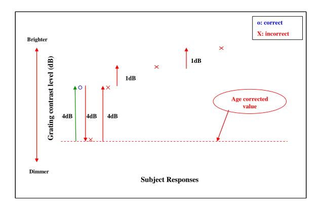
Figure 7.5 A schematic where, during the first reversal, four consecutive incorrect responses after the first correct response at the start value terminates the threshold sequence.
