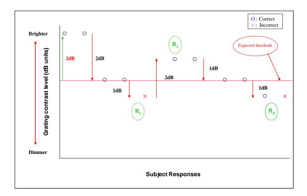
**Figure 7.17** A schematic of the staircase, for any one seed point, where 3 reversals determine the length of the staircase, and the final reversal is used to calculate the threshold (i.e., the average of the first incorrect and the last correct responses).
