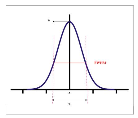
**Figure 5.1** A one-dimensional Gaussian function:  $\sigma$  is the Full Width at Half Maximum height (FWHM), a is the maximum height and x is the centre of the distribution.
