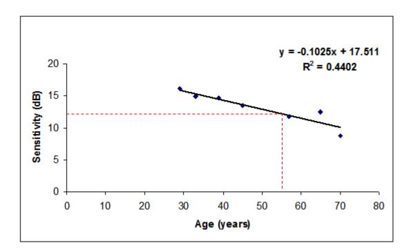
**Figure 7.9** The relationship between Michelson contrast, expressed as sensitivity in dB, against age and in the absence of the noise mask, for the seed point at  $+10^{\circ}$ ,  $+16^{\circ}$ . The dashed red line indicates, as an example, the 'start' value of 12dB for an individual aged 55 years.
