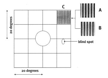
**Figure 1.2** The stimulus for the first generation Frequency Doubling Technology (FDT) perimeter. The 0.5 cycles per degree vertical sine wave grating, counterphased at 25Hz, embedded in a  $10^{\circ}$  x  $10^{\circ}$  square stimulus is illustrated at A, B and C. The circular stimulus at the centre has a diameter of  $5^{\circ}$  (Jampel et al., 2011).
