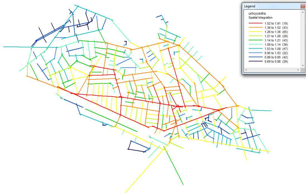
Figure 63 - Case study 1 – urban area cycle network including additional routes (global integration with route weightings)
