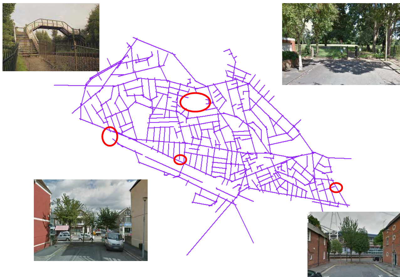
Figure 50 - Case study 1 - urban area. Example of connections available to cyclists that are inaccessible to motor traffic
