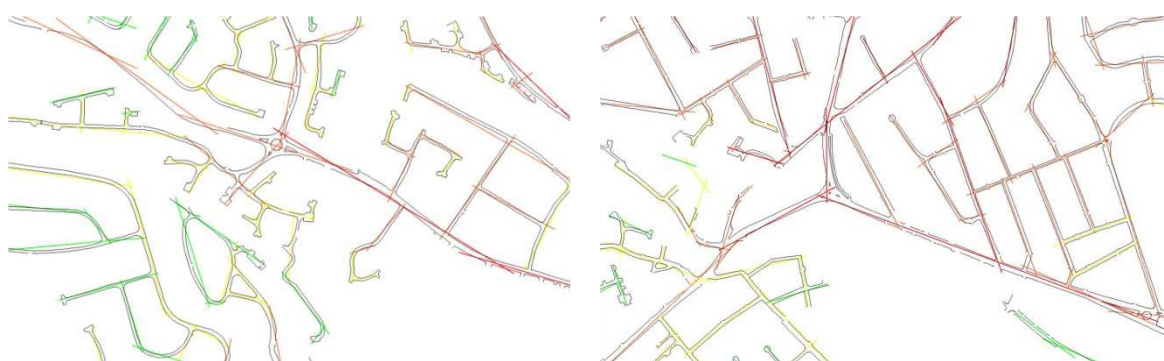
Figure 20 – Examples of axial line maps for different areas of a city (red lines indicate well integrated routes, green indicates less integrated routes)
