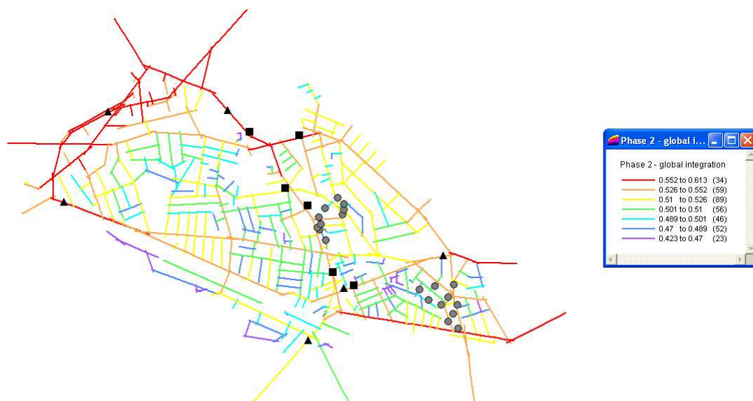
Figure 35 - Global spatial integration map for case study 1 - urban area when extracted from full Cardiff map
