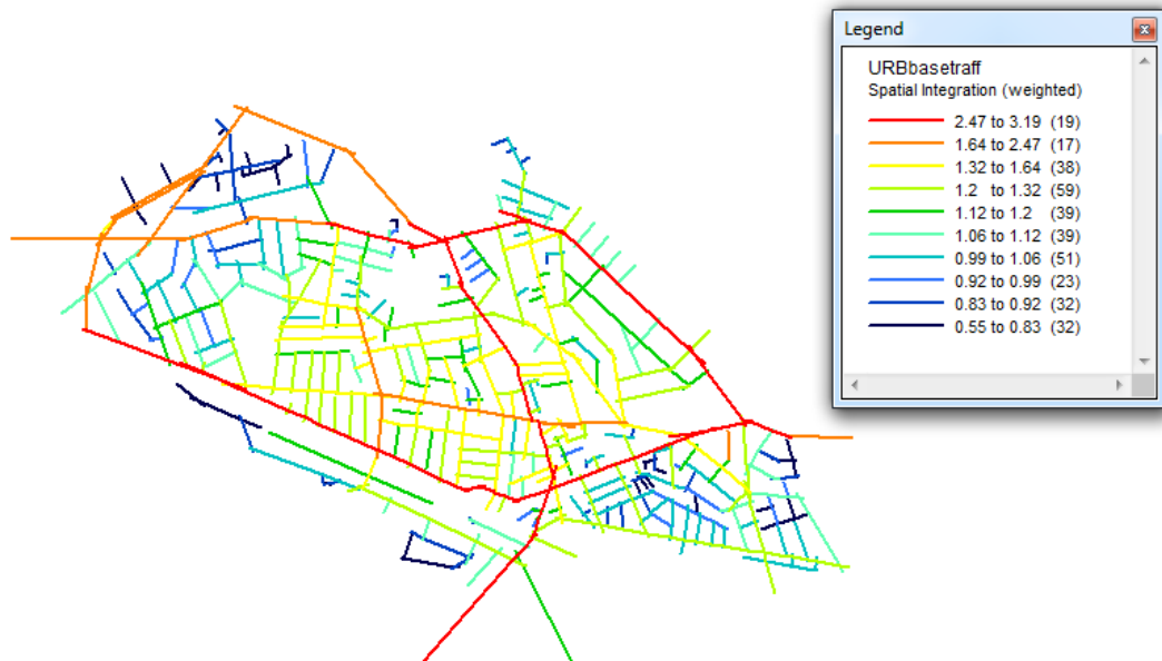
Figure 59 - Case study 1 – urban area motor traffic flow global integration with road weightings
