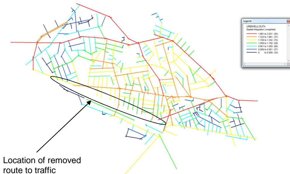
Figure 60 - Case study 1 – urban area motor traffic flow global integration with selected road removed to demonstrate the change in relative flow patterns as a result of motor traffic infrastructure changes
