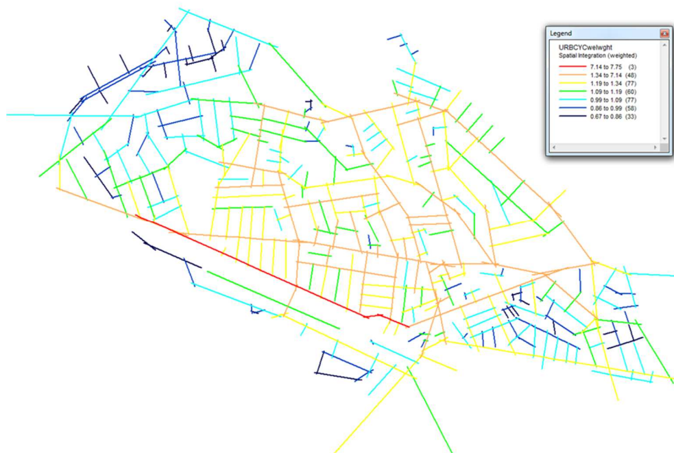
Figure 62 - Case study 1 – urban area cycle network global integration with weighting factor applied to motor traffic free route
