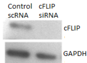
Figure 2.2: Optimisation of cFLIP antibody for Western blotting: MCF-7 cells were transfected with siRNA targeting cFLIP or a scrambled control siRNA: Inhibition of cFLIP reduced signal and confirmed antibody specificity
