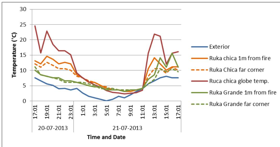
Figure 7: Simultaneous measurements of dry-bulb temperature and globe temperature at different points in plan. Ina Lewfu 20<sup>th</sup>-21<sup>st</sup> July 2013 (Austral Winter)
