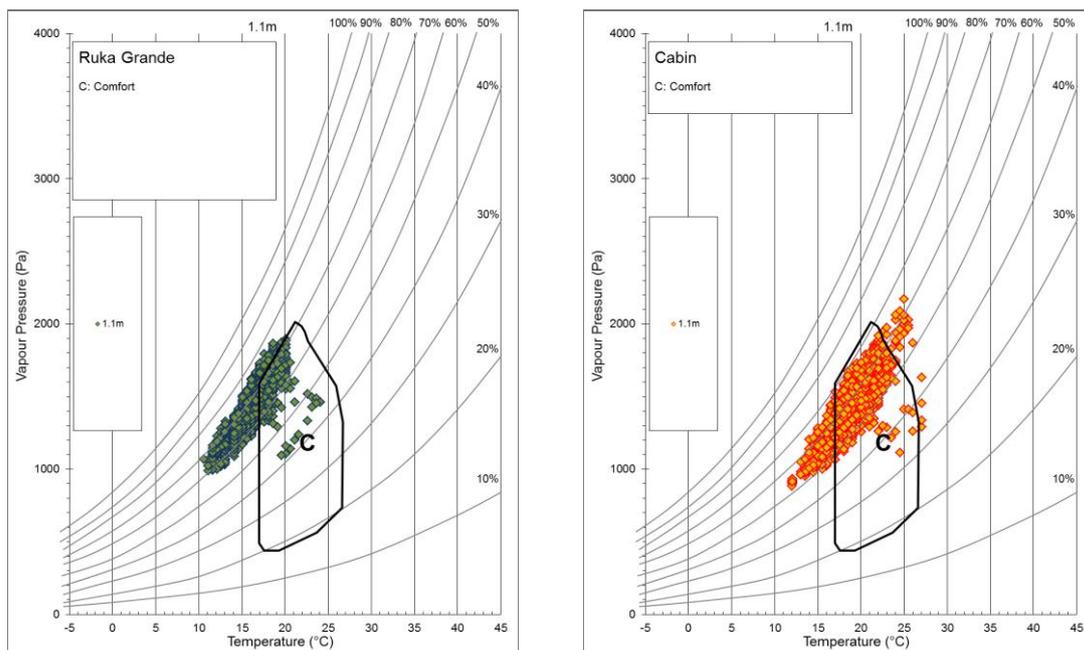
Figure 18 & Figure 19: Psychrometric charts showing temperature and relative humidity of the air in the *ruka grande* and timber cabin from 4<sup>th</sup> January to 26<sup>th</sup> February 2014 (Austral Summer)
