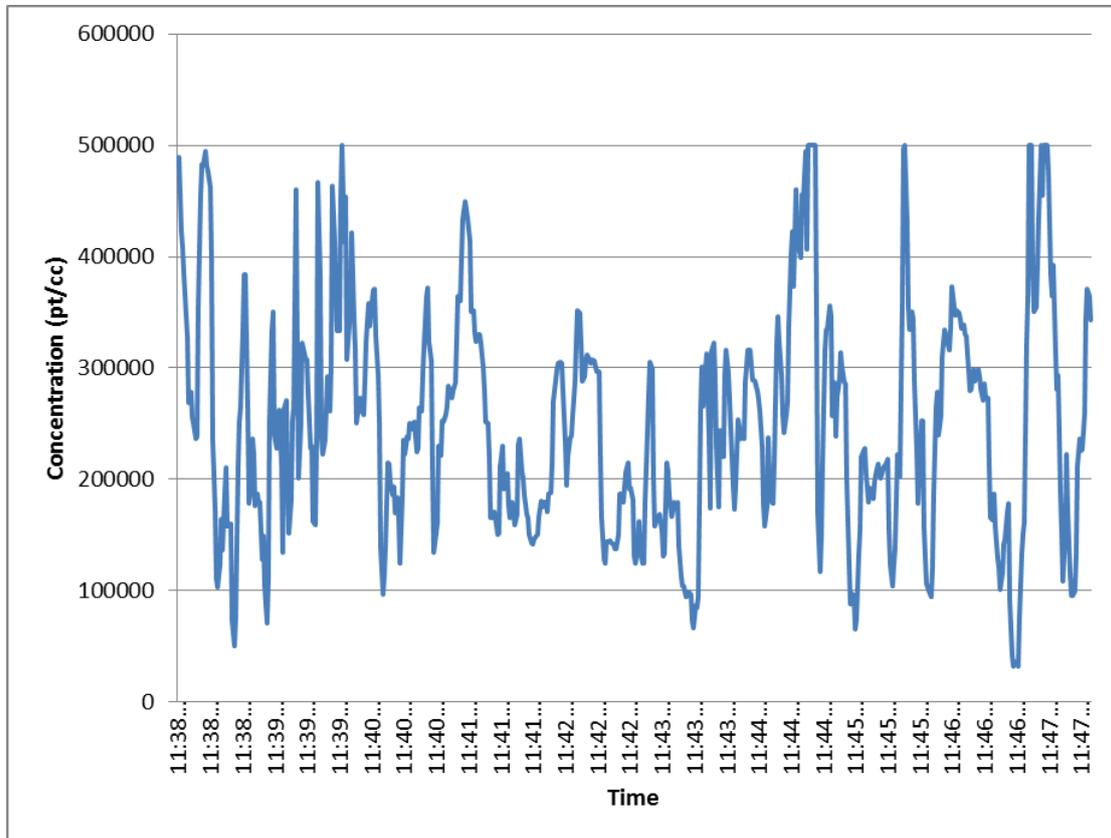
Figure 27: Measurements of concentration of ultra fine particulate matter in the *fogón* of Don Crescencio 25<sup>th</sup> July 2013 (Austral Winter) with open hearth lit.
