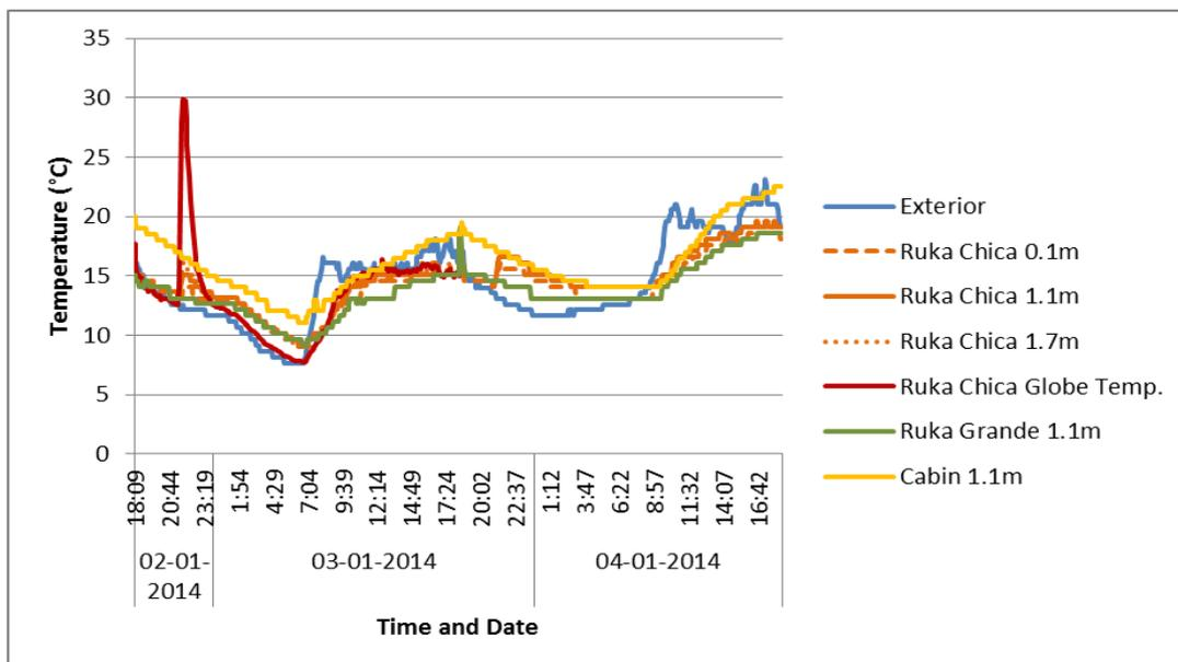
Figure 9: Simultaneous measurements of dry-bulb temperature and globe temperature. Ina Lewfu 2<sup>nd</sup>-4<sup>th</sup> January 2014 (Summer)
