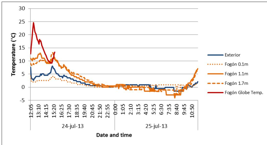
Figure 25: Simultaneous measurements of dry-bulb temperature and globe temperature at different heights. *Fogón* of Don Crescencio 24<sup>th</sup>-25<sup>st</sup> July 2013 (Winter)
