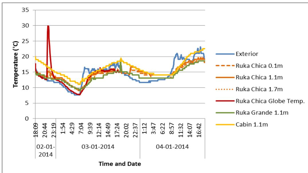
Figure 9: Simultaneous measurements of dry-bulb temperature and globe temperature. Ina Lewfu 2<sup>nd</sup>-4<sup>th</sup> January 2014 (Summer)
