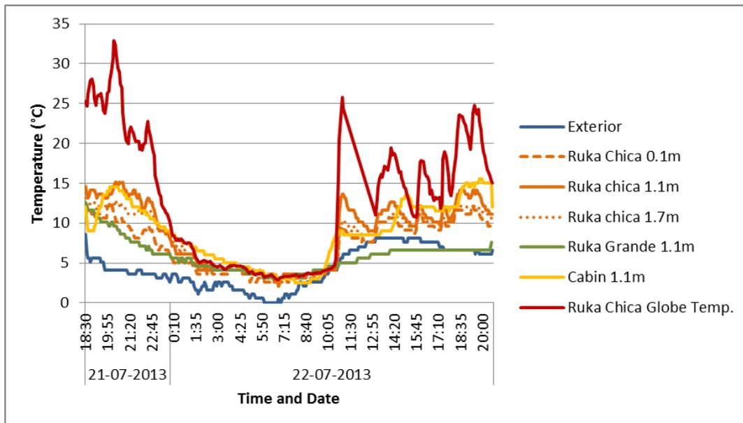
Figure 8: Simultaneous measurements of dry-bulb temperature and globe temperature. Ina Lewfu 21<sup>st</sup>-22<sup>nd</sup> July 2013 (Austral Winter)
