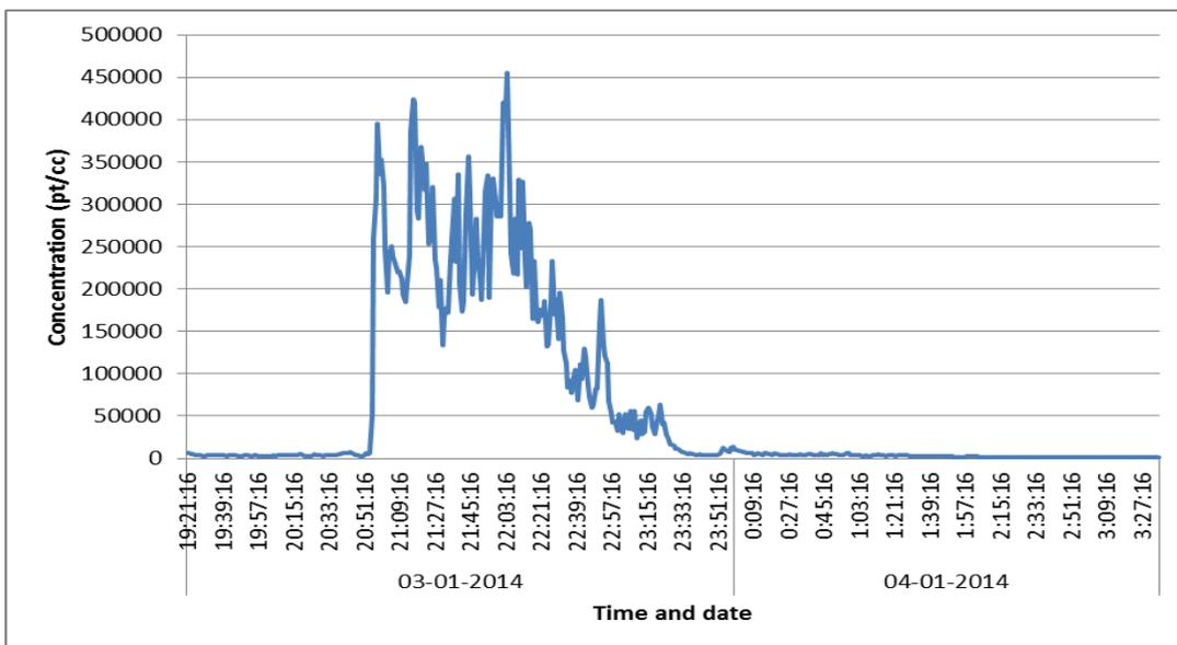
Figure 11: Measurements of concentration of ultra fine particulate matter in the ruka chica, Ina Lewfu 3<sup>rd</sup>-4<sup>th</sup> January (Austral Summer).
