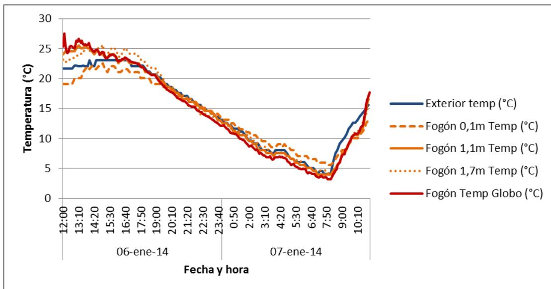
Figure 26: Simultaneous measurements of dry-bulb temperature and globe temperature at different heights. *Fogón* of Don Crescencio 6<sup>th</sup>-7<sup>st</sup> January 2014 (Austral Summer)
