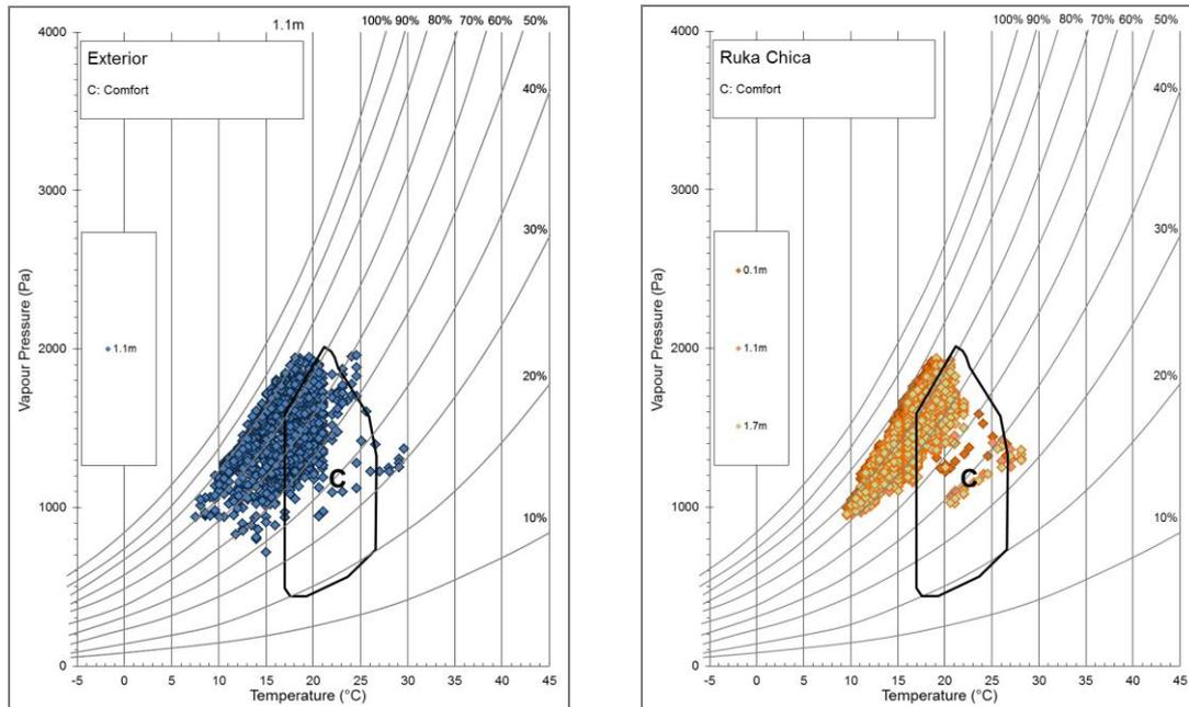
Figure 16 & Figure 17: Psychrometric charts showing temperature and relative humidity of the air externally and in the *ruka chica* from 4<sup>th</sup> January to 26<sup>th</sup> February 2014 (Austral Summer).
