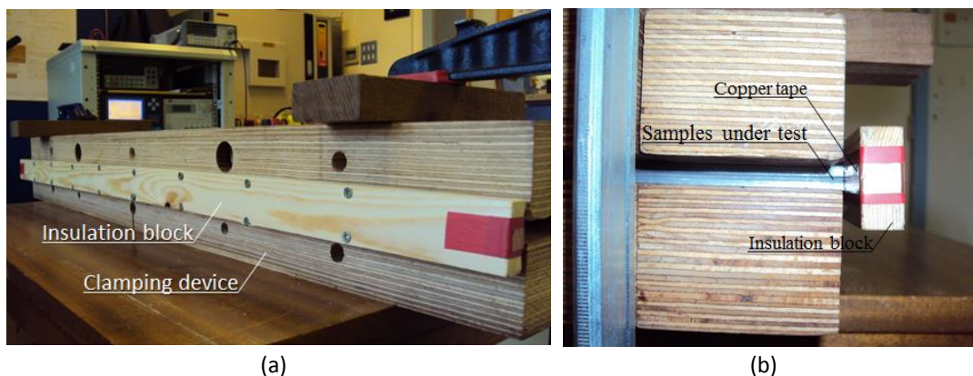
Fig 8-18 Experimental set-up after applying artificial short on one side of the stack
