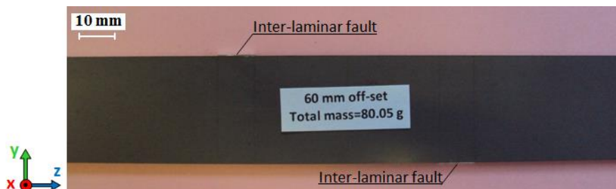
Fig 7-17 (a) Side view and (b) top view of a stack of four laminations with an inter-laminar short circuit with axial off-set position
