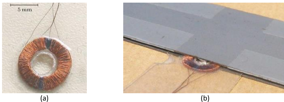
Fig 3-31 (a) Top view of a Rogowski coil (b) Application of a Rogowski coil to measure inter-laminar fault current between two laminations [3.18]
