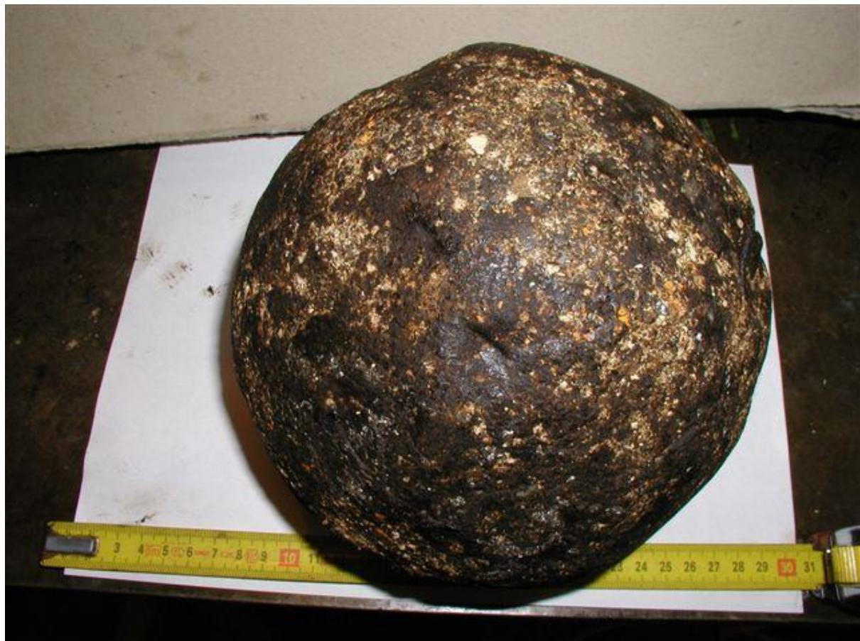
**Figure 15 A Sludge Ball Filtered from a Chilled Water System**
