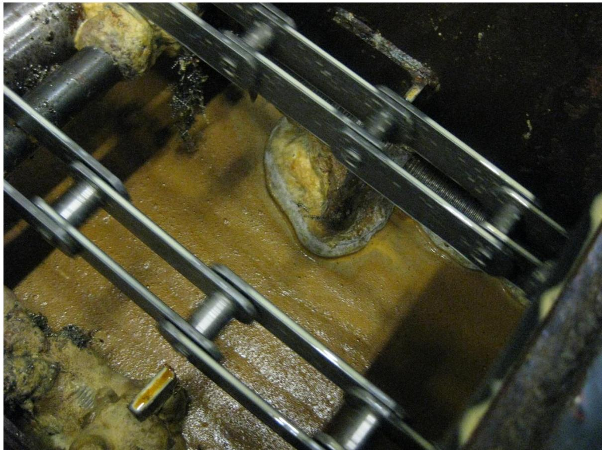
**Figure 12 Suspected Biofilm in the Swarf Removal Trenches**
