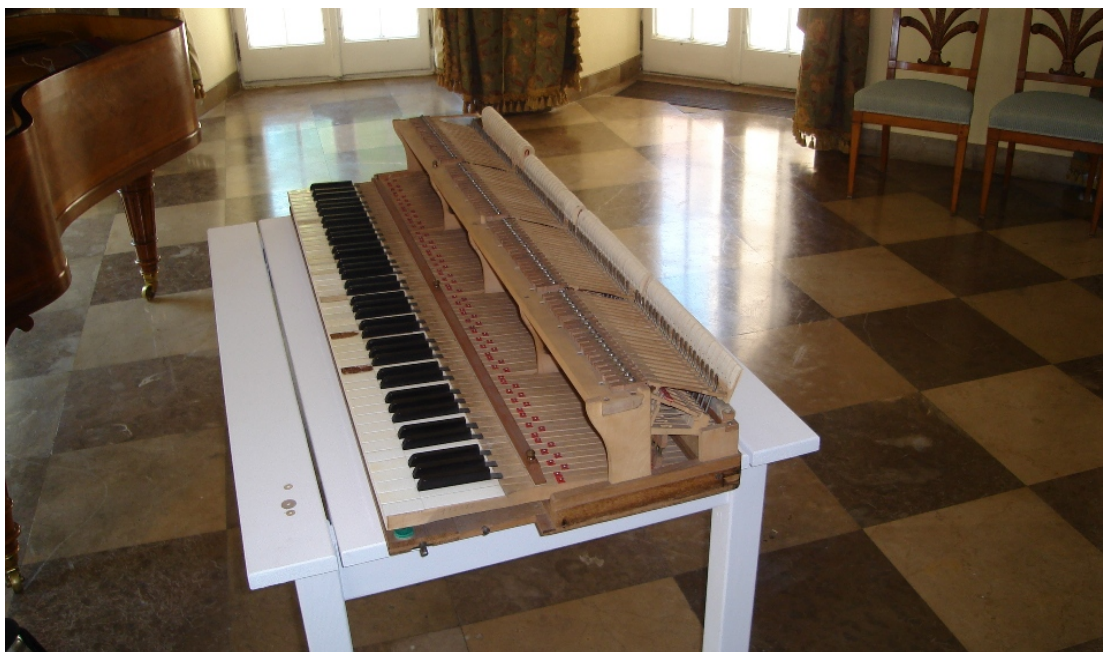
Fig. 20. The action of Érard piano with a pencil marking of its serial number and also with a surname – Vigin (the piano tuner who changed the hammers in February, 1934). Photos: J. Walczak.
