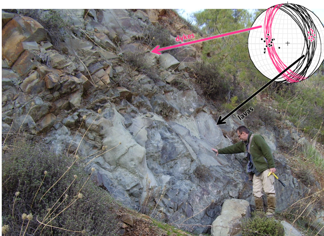
Figure 3.33 Basal Group out crop at Agia Koroni. Large pillow lavas (1.5m) in the lower half of photo are pale green and dipping to the right (plotted in black on stereonet). Dykes are grey-brown in upper part of photo, dipping to the left, (plotted in pink).
