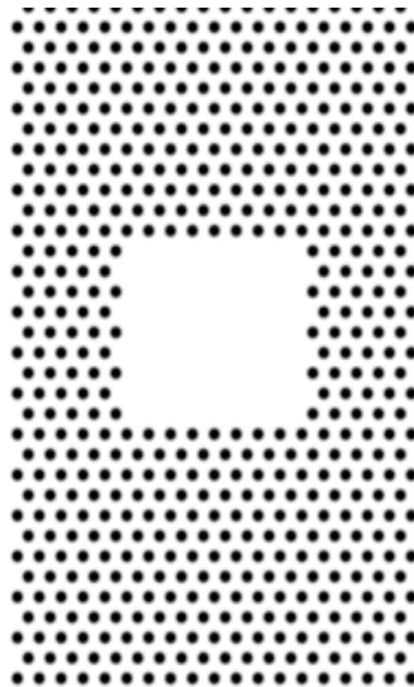
Figure 3.5: Schematic of lattice with a hole introduced of size x=8 and y=4 , placed at the centre of the lattice
