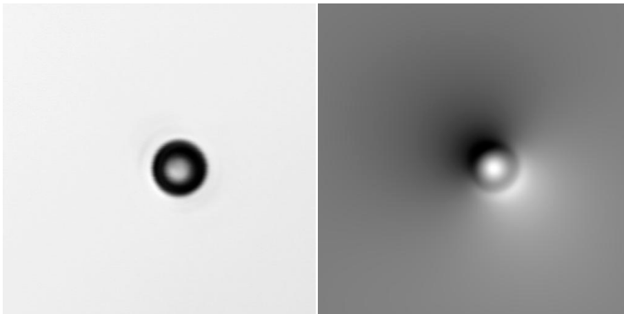
Figure 2.3: Bright field image of a 15µm polystyrene bead obtained from laser scanning microscopy (left) and the phase image that was produced using it (right). An obvious asymmetry was observed in the phase image, which was initially thought to be caused by Brownian motion during image acquisition.
