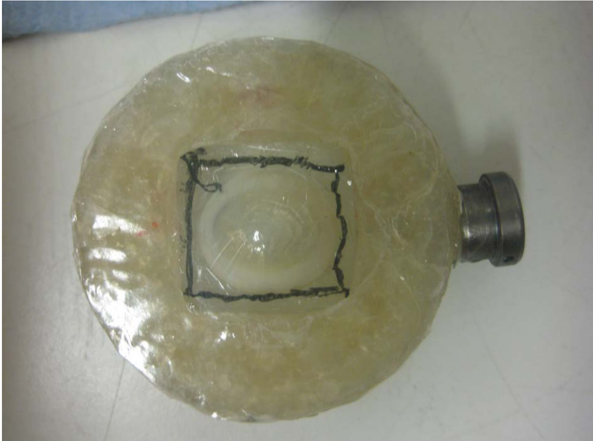
Figure 4.4: Image showing tissue from right eye within a holding case that was used during x-ray diffraction pattern acquisition. Tissue was wrapped in conventional wrapping film (polyvinylidene chloride) to prevent dehydration.
