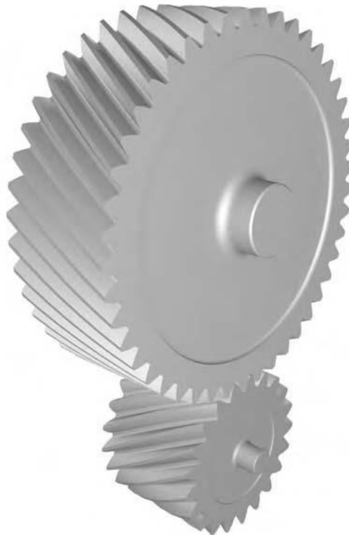
Figure 1.2: A Pair of helical gears in contact (Litvin & Fuentes, 2004).
