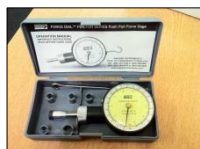
Figure 3: Manual algometer used to measure Pressure Pain Threshold (PPT) at 3 different sites
