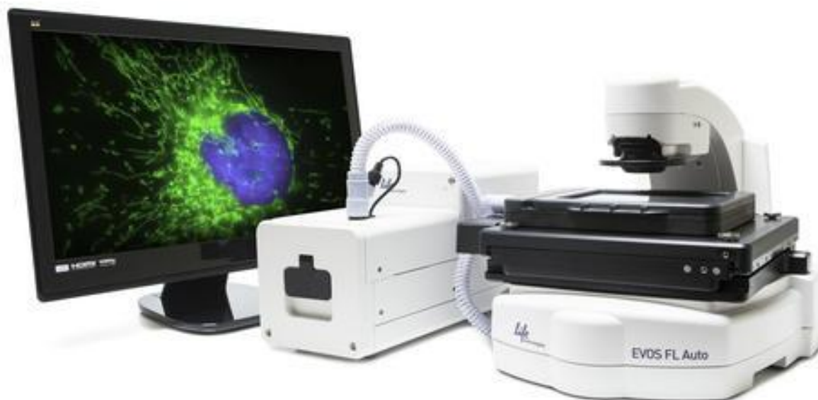
Figure 2.9 EVOS system used in cell migration study.
