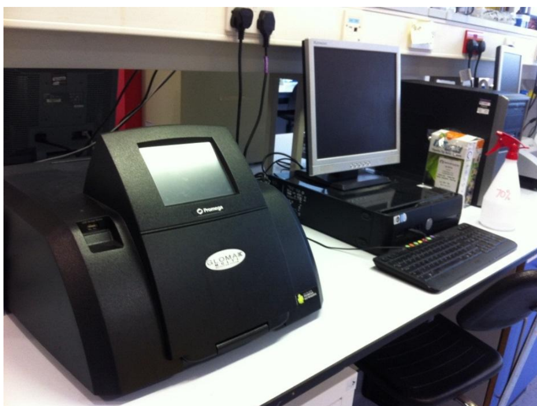
Figure 2.8 Multiple plate reader.
