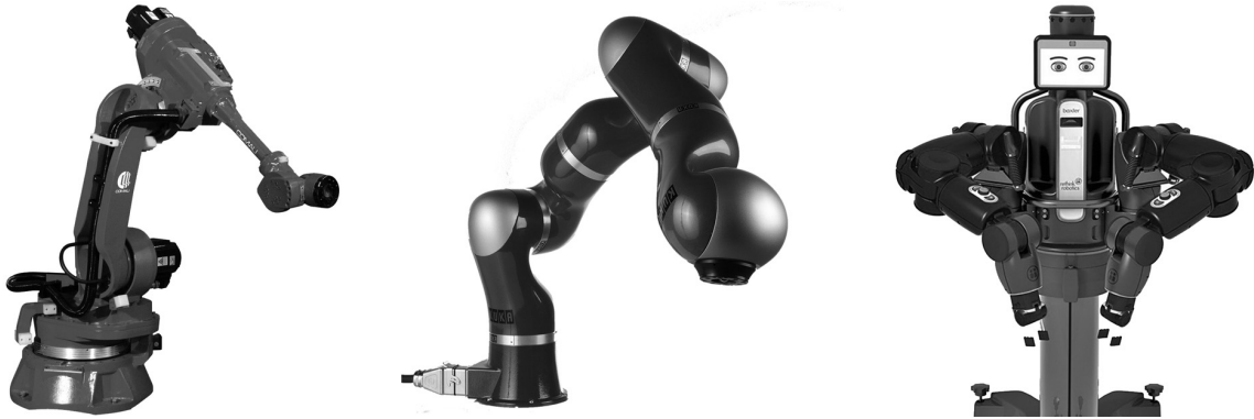
▲ Figure 10. Left: Typical industrial robot. [5] Middle: KUKA LWR. [5] Right: Baxter. [44].
