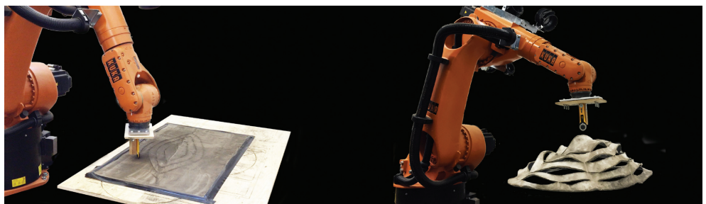
► Figure 15. Left: Setup and end effector for robotic cutting of concrete impregnated fabric. Right: 1.0x0.7x0.7 popped-up prototype.
