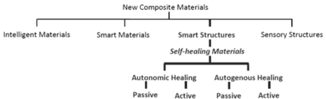
Figure 2.2 – Tree diagram highlighting new advanced composite materials (Dunn 2010)
