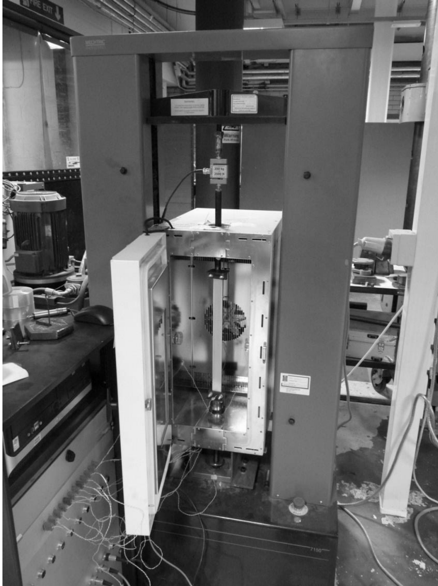
Figure 3.8 – Experimental setup for heat-activated stress relaxation tests
