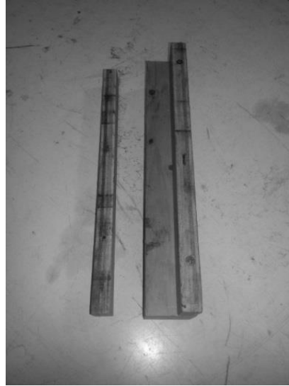
Figure 3.2 – Timber jig used to hold strips while grips were attached
