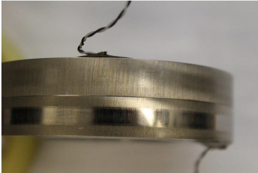
Figure 5-31 Close-up photograph of hard disk (upper) and soft disk (lower) beside one another following removal from their respective test shafts
