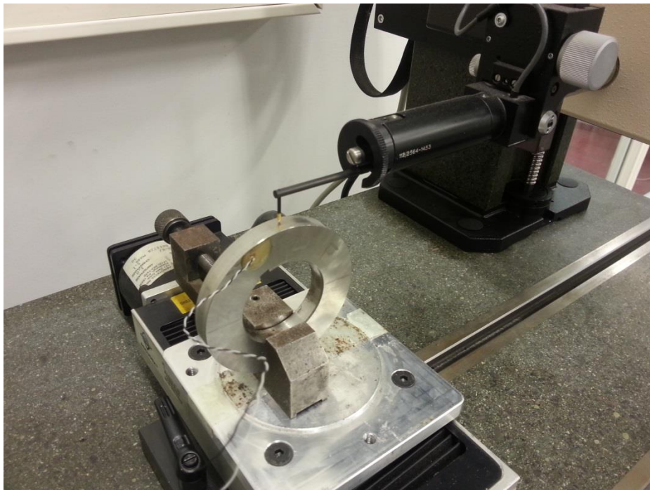
Figure 6-2 Test disk positioned on Talysurf stage
