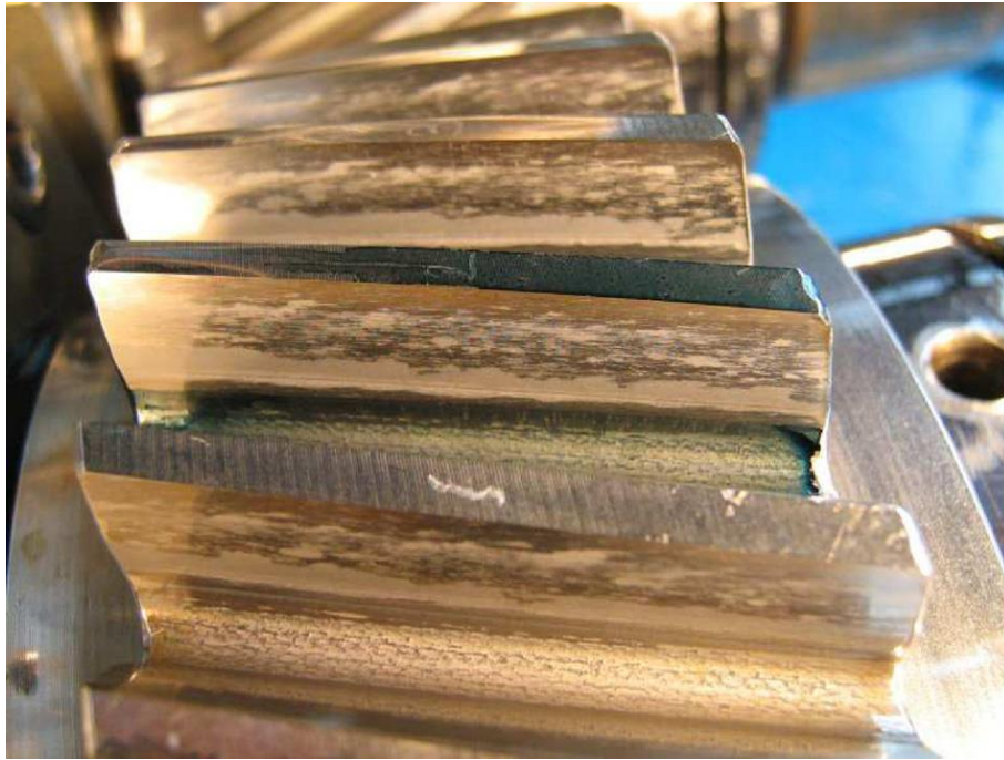
Figure 1-13 Photograph of helical gear with micropitting visible as matted region on dedendum of teeth (Evans et al., 2013)
