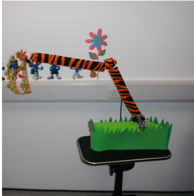
Figure 3.5. Customised child-friendly head stabiliser.
