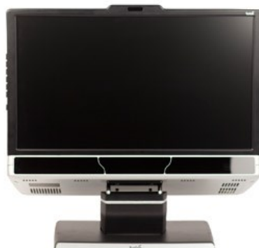
Figure 3.1. Tobii TX300 infrared eye tracker unit attached to the widescreen monitor (Tobii Technology 2015a).
