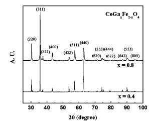
FIG. 1. X-ray diffraction data for polycrystalline cobalt ferrite samples with compositions of  $CoFe_{2-x}Ga_xO_4$  (x=0.4 and x=0.8).
