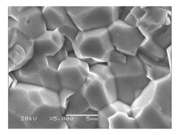
FIG. 2. SEM image showing a homogeneous, equiaxed microstructure of the  $CoFe_{2-x}Ga_xO_4$  with x=0.8.
