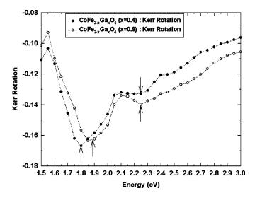
FIG. 3. Magneto-optic Kerr rotation spectra for  $CoFe_{2-x}Ga_xO_4$  (x=0.4 and x=0.8) samples.
