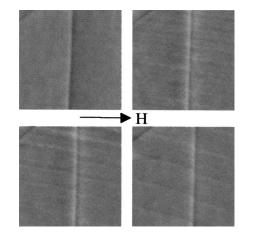
FIG. 3. Magnetic force images of junction and electrode at, from left to right and top to bottom, 100, 400, 200, and a return to 0 Oe. Images are also in chronological order.
