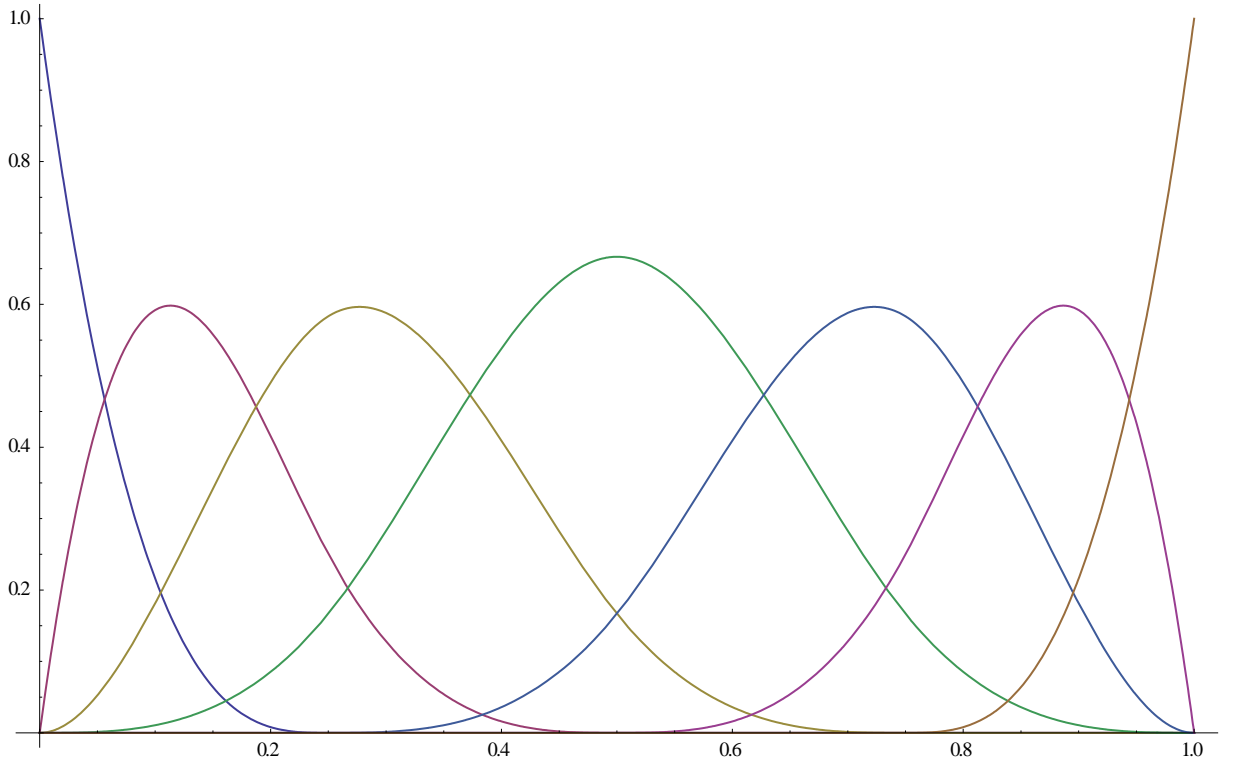
Figure 16: B-Spline basis function over the knot vector \{0, 0, 0, 0, 0.25, 0.5, 0.75, 1, 1, 1, 1\} .
