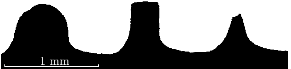
Figure 49: Tools measured before machining.
