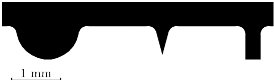
Figure 46: The three shapes used in the validation of the roughness and machining gap models.
