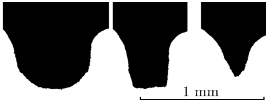
Figure 50: Tools measured after machining.
