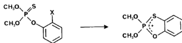
Fig. 3. MS fragmentation of ortho -substituted compounds to produce m/z 217 ( X = \text{Cl, Br, I, NO}_2, \text{CH}_3\text{SO or CH}_3\text{SO}_2 ).
