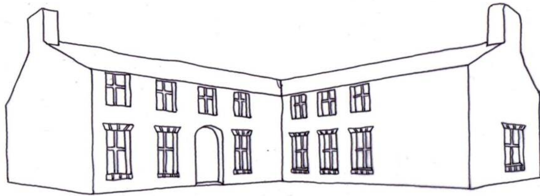
Figure 22: Phase 5 saw the upper house have several windows blocked-up due to the introduction of the window tax and the use of part of the great hall as a cow shed. Ceri Leeder.
