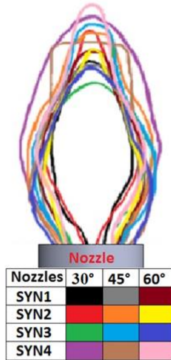
Figure 5-22: CFD results of CRZ size
