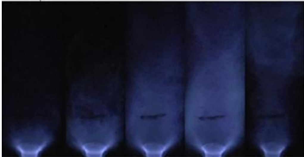
Figure 5-15: Pulsating flame. Progression of LBO seconds before final onset. S = 1.05 , \Phi = 0.525 . Frequency = 10 Hz
