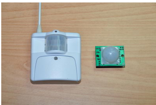
Figure 4.46: Wireless presence sensor in dwelling 6
