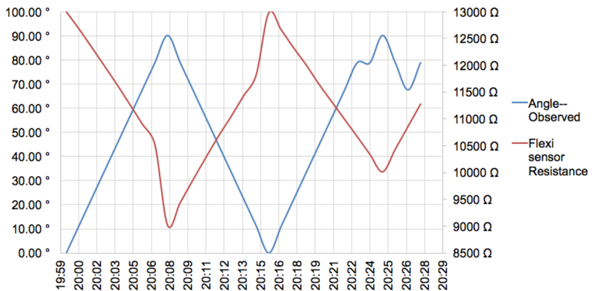
Figure 5.49: Comparison of observed and measured door angle, Flexi sensor
