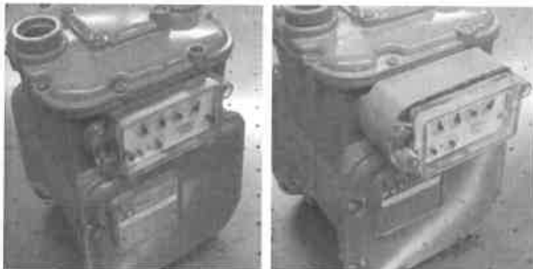
Figure 2.17: Retrofit assembly & attachment to meter.
