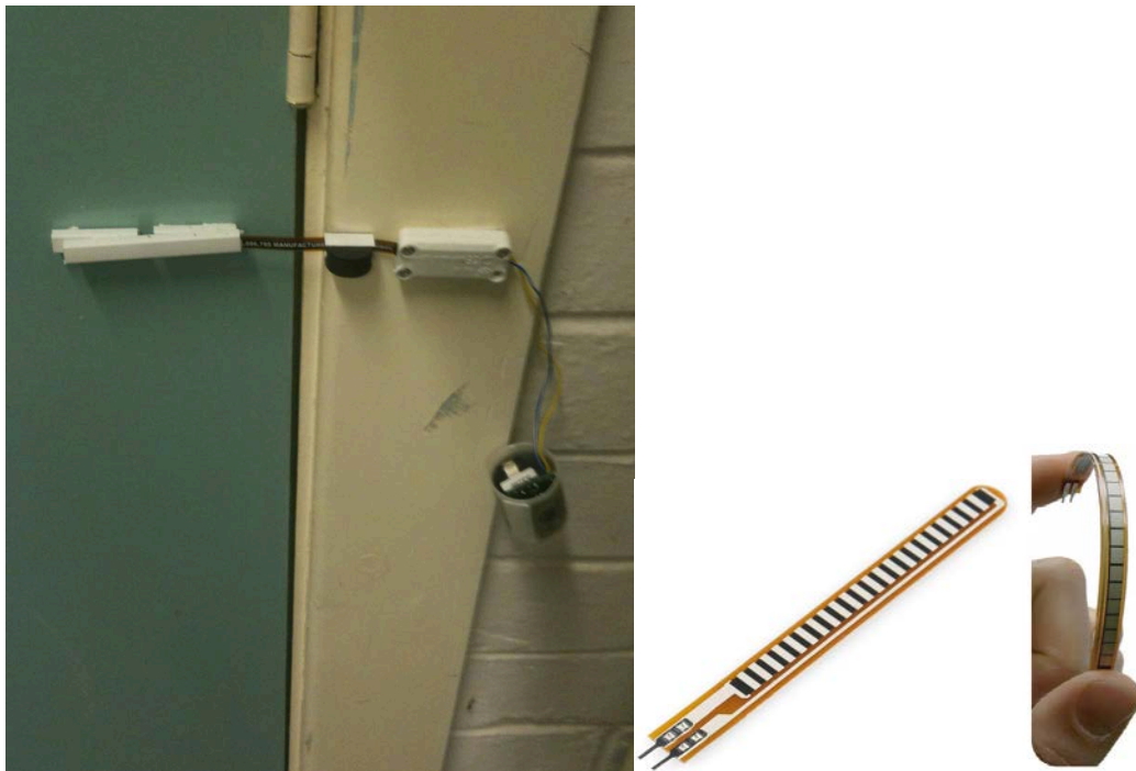
Figure 3.18: Rotary resistor angle measurement on a door
