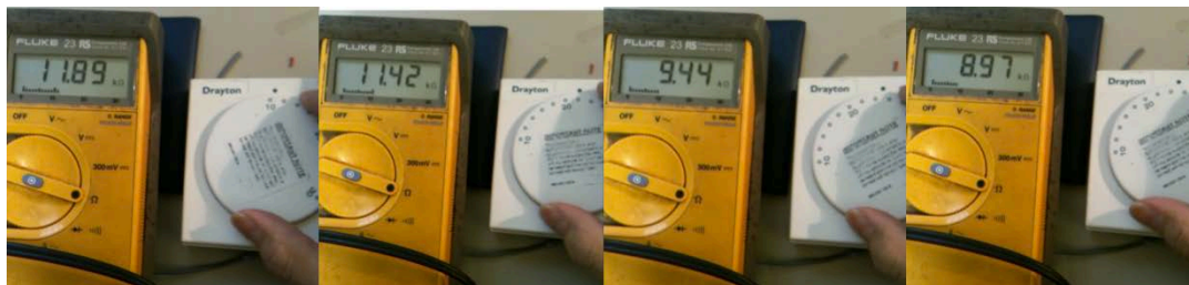
Figure 3.7: Thermostat internal resistant value variation
