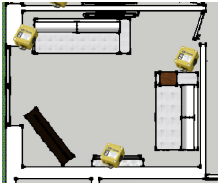
Figure 5.57: Different locations temperature humidity logger in living room –dwelling 6, top left: near window, top right: near entrance, bottom: fireplace
