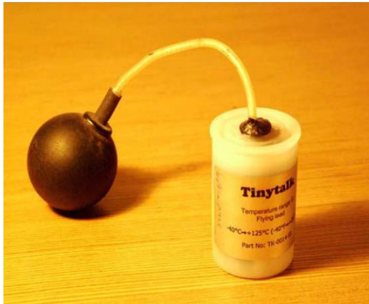
Figure 3.36: Gemini Tinytalk Data Logger. Source: author.
