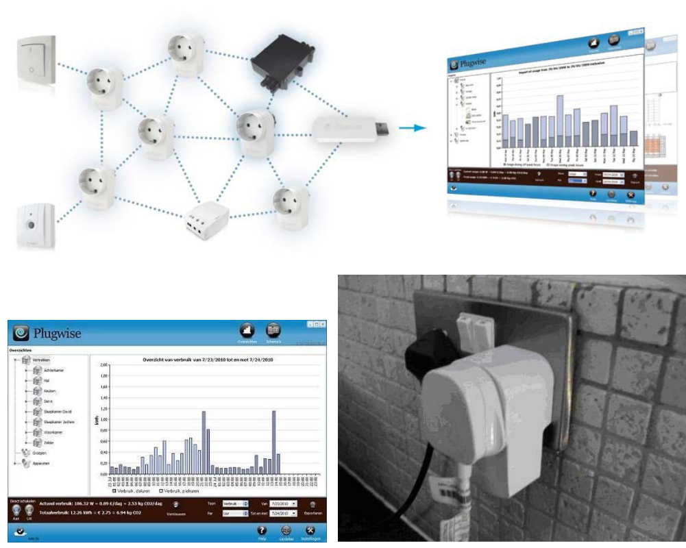
Figure 3.35: Plugwise home appliance monitoring set up
