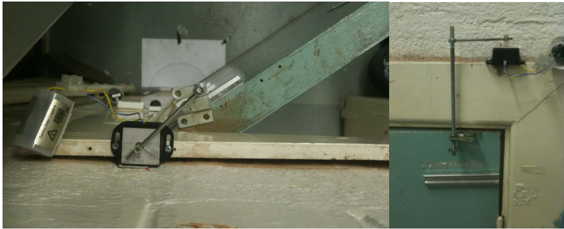
Figure 3.18: Rotary resistor angle measurement on a door
