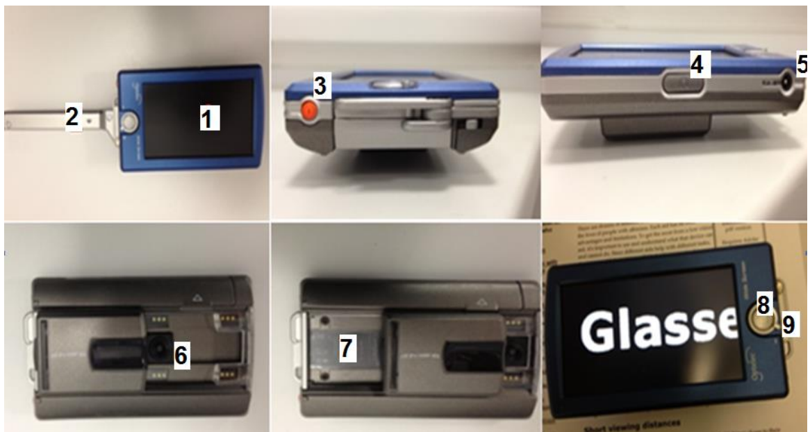
Figure 3.2: A PELVA (Compact+) incorporates: 1) a display screen, 2) a collapsible handgrip, 3) an on/off switch, 4) a snapshot button to freeze an image on the display screen temporarily, 5) a power adaptor for rechargeable batteries, 6) a camera unit: auto-focus camera, 7) a battery compartment, 8) a mode button for a contrast viewing mode selection (e.g. a black letter on a white background or a white letter on a black background), and 9) a magnification dial: a control to change magnification levels.
