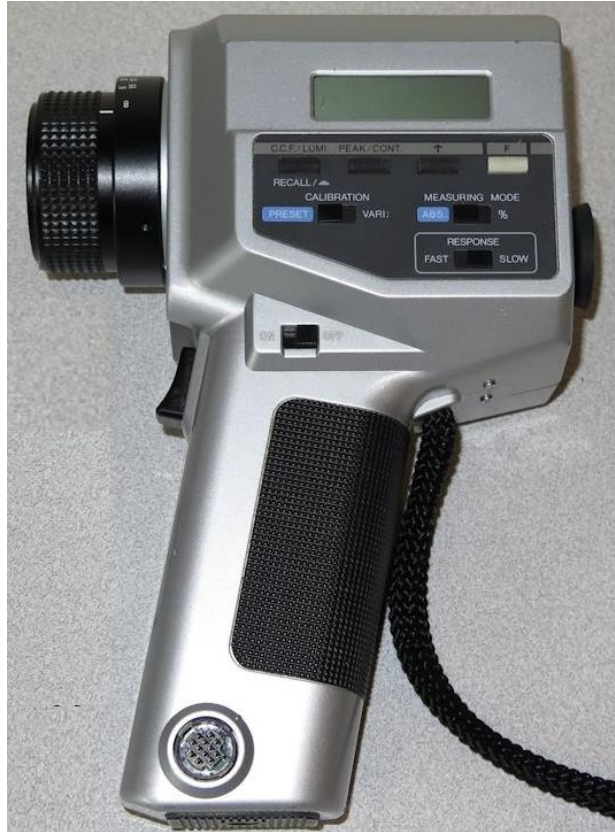
Figure 4.2: Konica Minolta LS-100 luminance meter (Konica Minolta INC, 2015).
