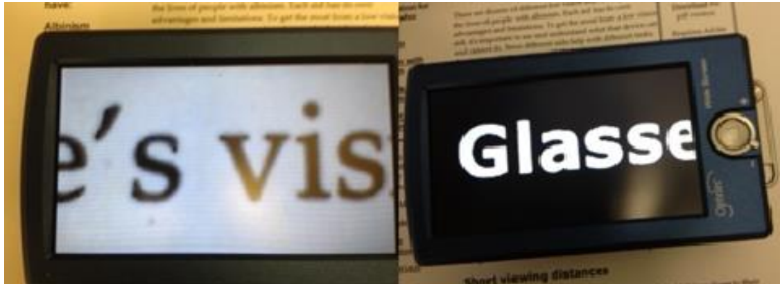
Figure 3.1: A PELVA (Compact+) is used by people with visual impairment to magnify a text or an object and to enhance contrast. The image contrast relationship is the same as the target; in the example a black target on a white background (Left). The image contrast relationship is opposite to the target (contrast reverse); in this example a white target against a white background (Right).
