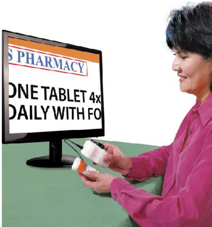
Figure 2.6: A mouse video magnifier. The camera is incorporated within the mouse that can be attached to a computer or TV screen [Max mouse electronic magnifier, Enhanced Vision – USA, cost (not including the screen): £125] (Enhanced Vision, 2015).
