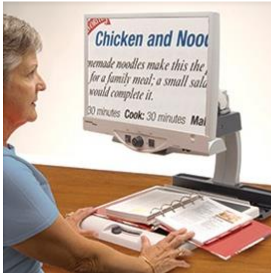
Figure 2.3: A desktop electronic magnifier (Merlin LCD desktop electronic magnifier/ Enhanced Vision – USA, cost: £1,766). It has a display screen and a moveable reading table (platform) (Enhanced Vision, 2015).
