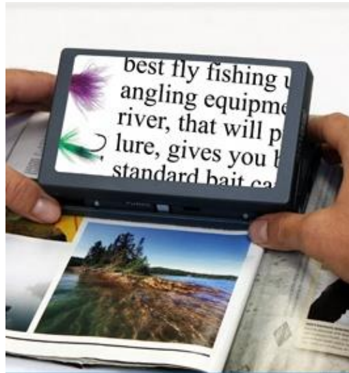
Figure 2.7: A pocket and portable electronic magnifier. It has a small display screen with few buttons (Amigo portable electronic magnifier, Enhanced Vision – USA, cost: £930) (Enhanced Vision, 2015).
