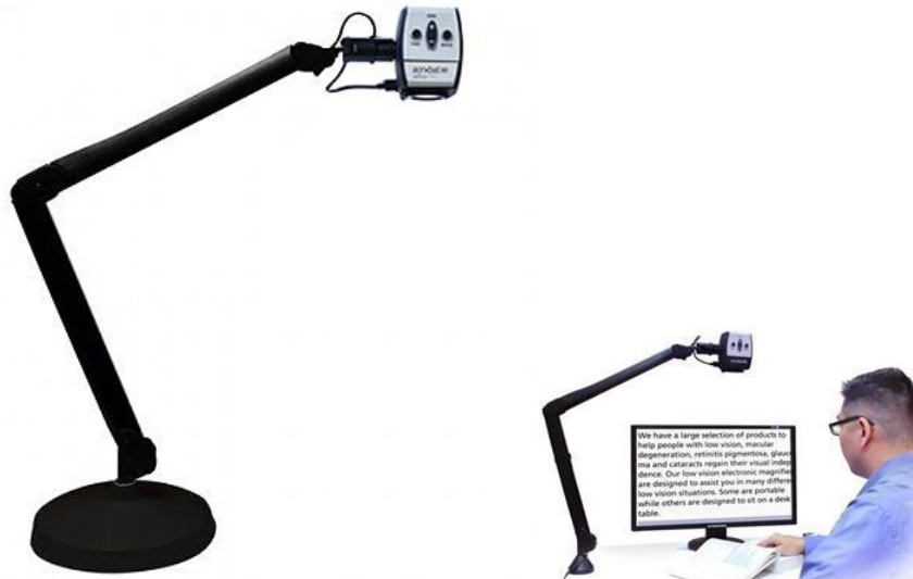
Figure 2.4: A flex-arm electronic magnifier with a computer display and a camera housed in a flexible arm (Acrobat HD ultra-long arm/ Enhanced Vision – USA, cost: £1,307) (Enhanced Vision, 2015).
