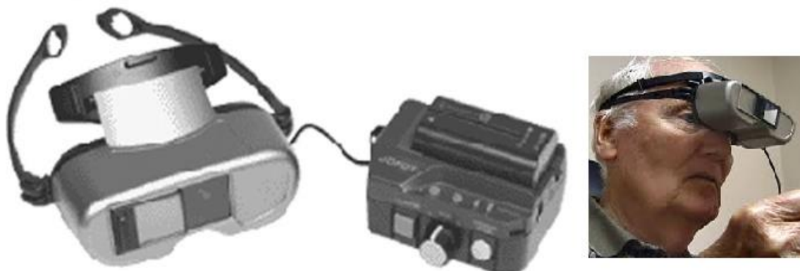
Figure 2.5: A head-mounted electronic low vision aid with camera incorporated on a head-mounted unit (Jordy head-mounted electronic magnifier, Enhanced Vision – USA, cost: £1,831) (Enhanced Vision, 2015).
