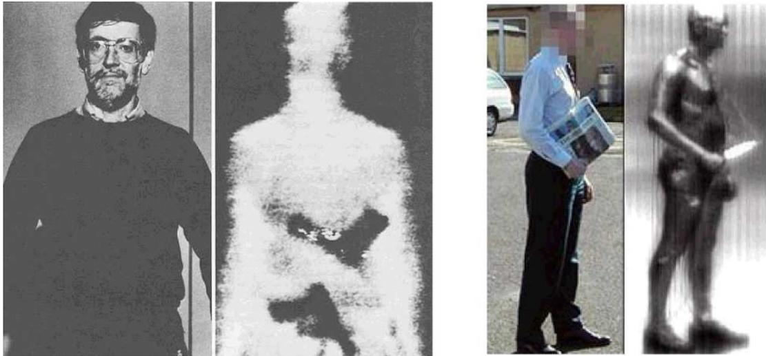
Figure 1.3: *Passive imaging for security applications: The left image is from the passive mm-wave imaging system from Millitech in 1995 and took 30 minutes to acquire with a single pixel 94 GHz Schottky diode heterodyne receiver. The image on the right was taken with a similar passive mm-wave scanner from QinetiQ in the mid 2000s. Image sources: Airline Passenger Security Screening, National Academies Press [National Research Council, 1996], and [Appleby et al., 1994].*
