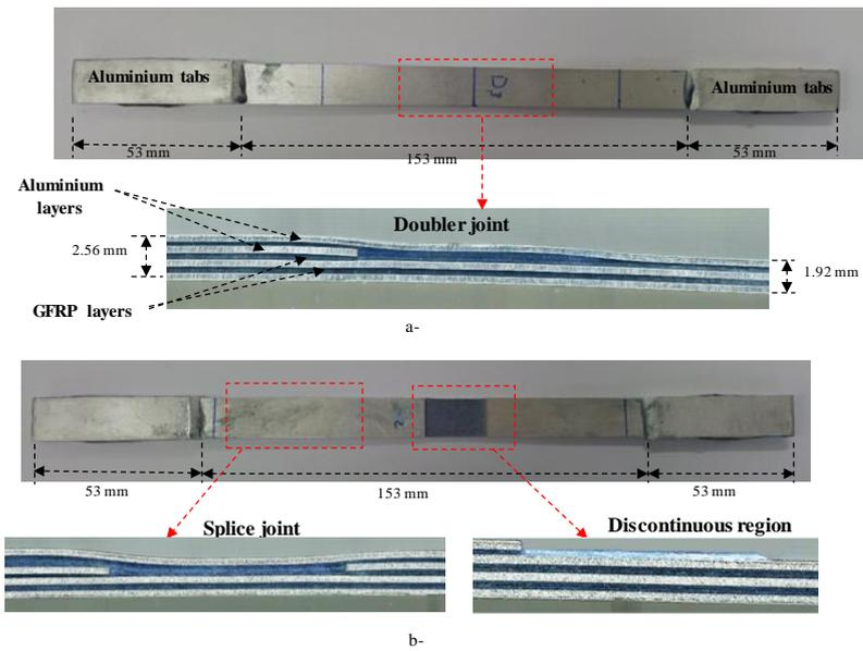
Figure 1. Specimen design for a) doubler b) splice
