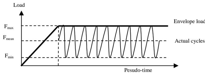
Figure 6. Schematic of fatigue modelling envelope load
