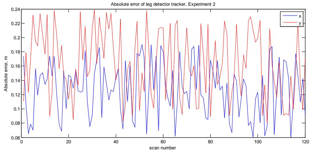
Figure 9-6: Leg detector experiment with two people at the opposite end of the room
