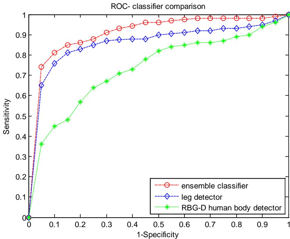
Figure 4-29: Comparison between the ROC curves of the classifiers
