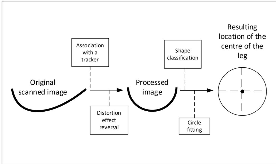
Figure 4-5: Overview of the laser scanned images processing
