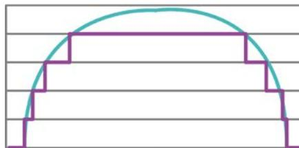
Figure 4-8: Illustration of the quantization effect of the sensor
