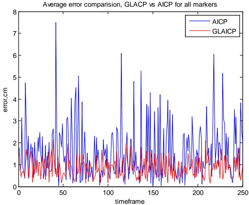
Figure 5-11: Distance average error comparison between GLAICP and AICP algorithms
