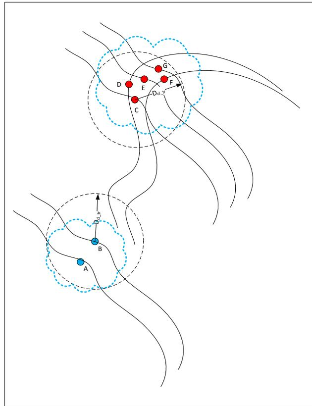
Figure 6-11: Proximetrics based clustering of states of the tracks
