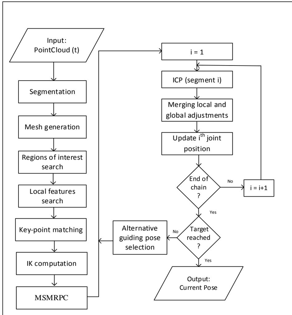
Figure 5-9: The GLAICP algorithm
