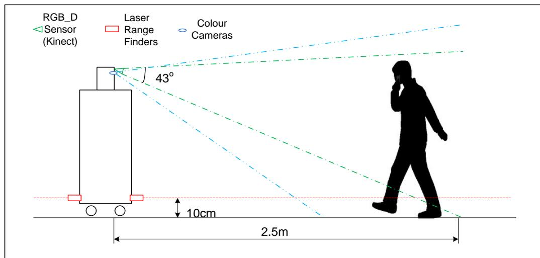
Figure 3-1: Experimental sensor spatial configuration – vertical field of view
