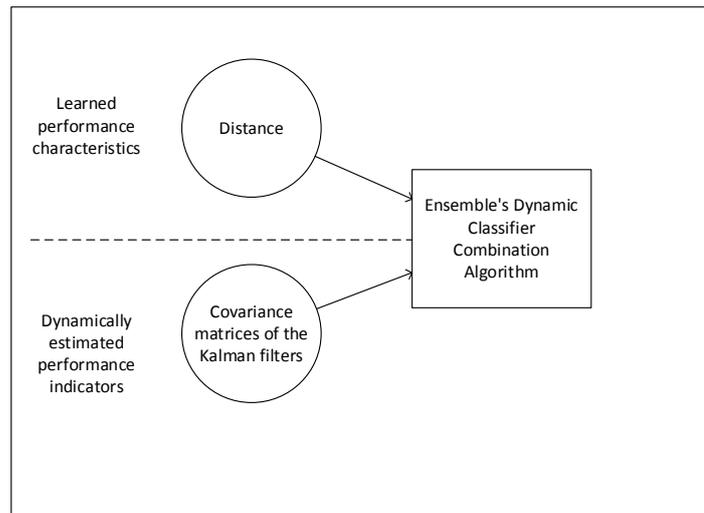
Figure 4-20: The concept of the two tier gating procedure for weighting of the classifiers in the ensemble
