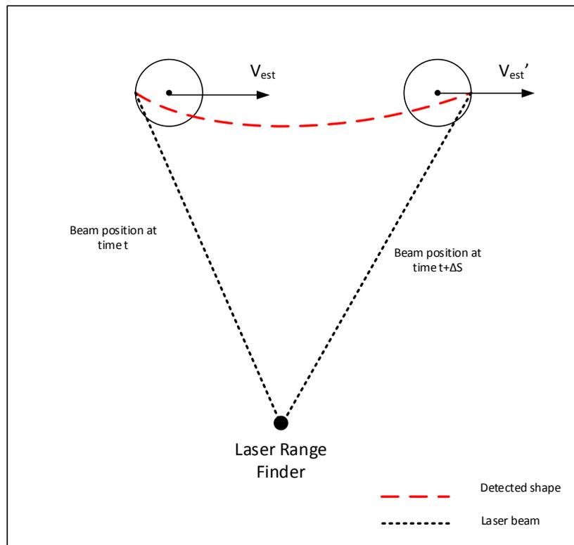
Figure 4-3: The distortion of the scan image caused by time delay between laser beams detecting points at different times
