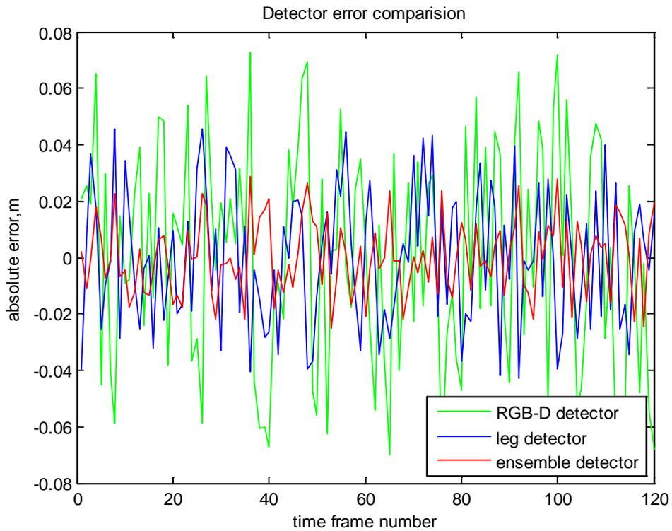
Figure 4-30: Error comparison between the leg, RGB-D and the ensemble detectors
