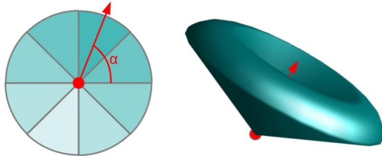
Figure 4-12: Division of space into cones for HISP computation
