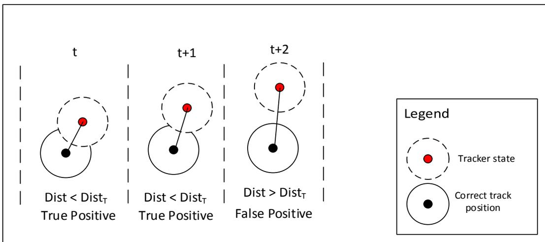
Figure 6-21: Determining true positive and false positive tracking results
