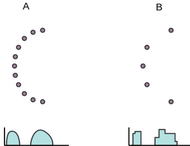
Figure 4-17 The effect of the detection distance on the signature. Displayed are the point cloud and the resulting signature: case A) at short distance; case B) at long distance
