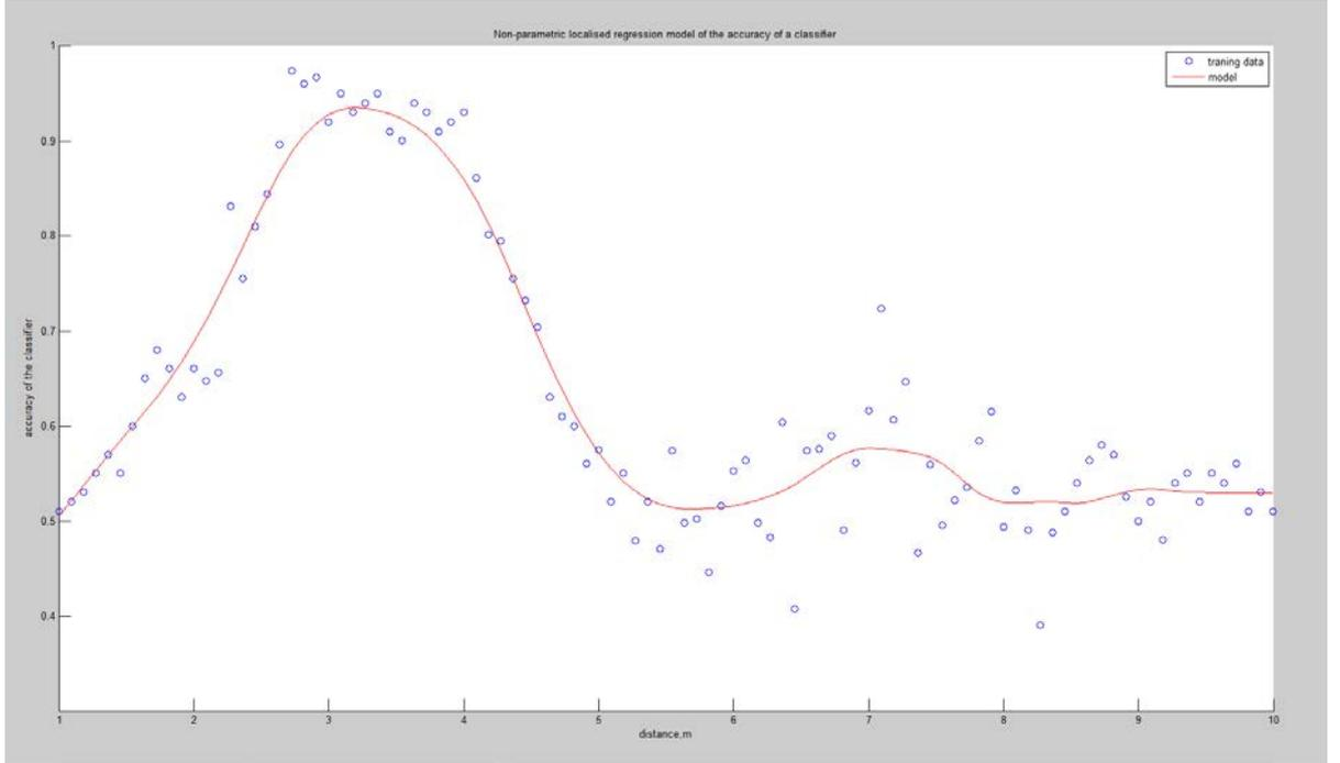
Figure 4-21: Typical distribution of the accuracy of a classifier over distance and the localised regression smoothing model
