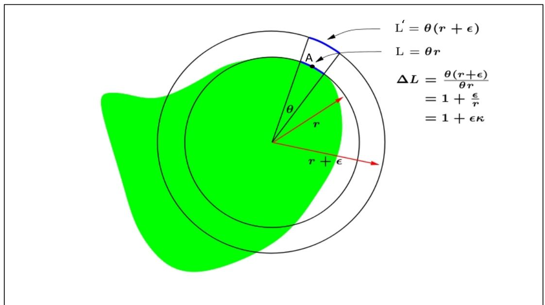
Figure 9-3: Curvature at a point of a curve
