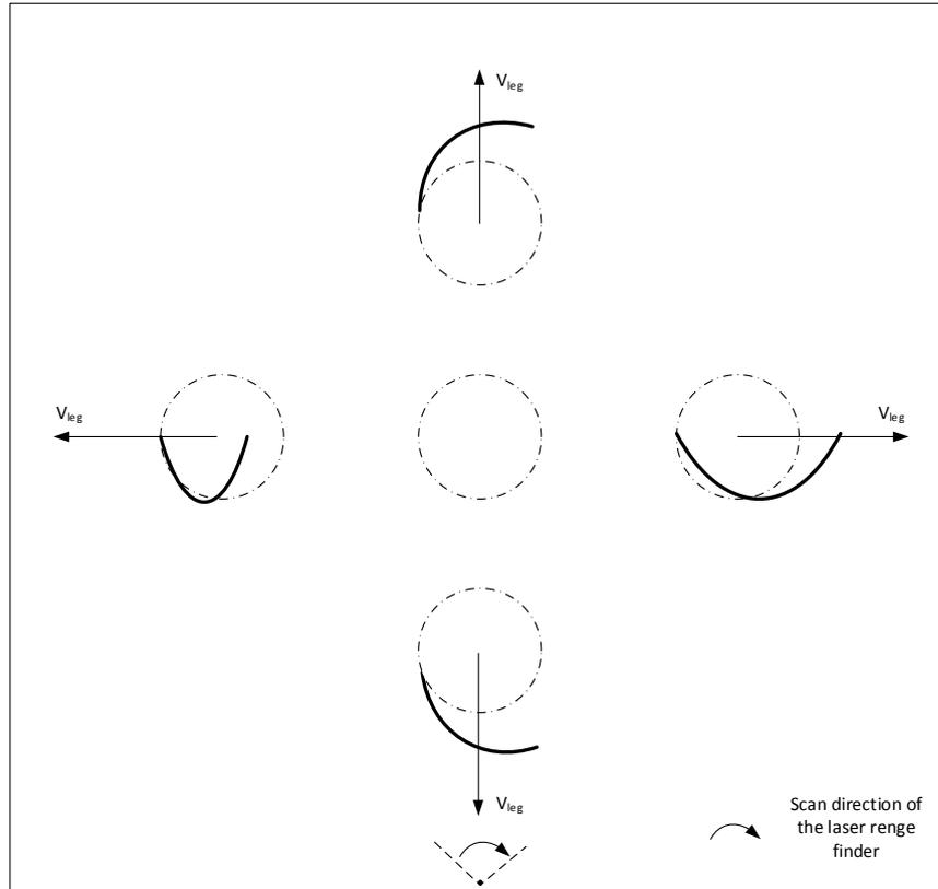
Figure 4-4: Illustration of the shape distortion of a moving leg in different directions
