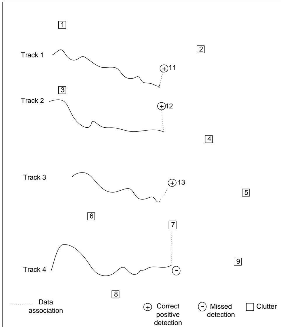
Figure 6-4: Example of tracks, observations, detections and possible associations
