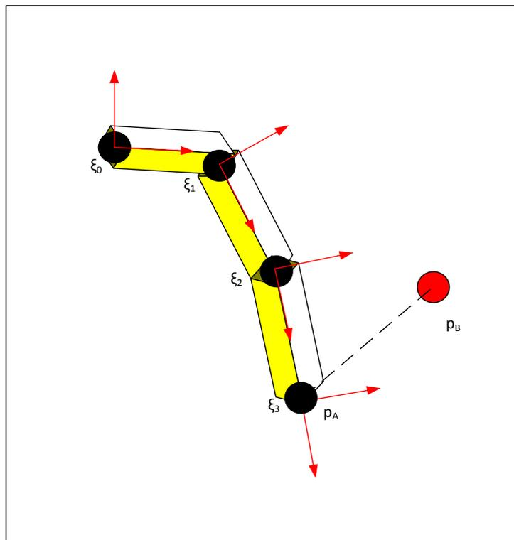
Figure 5-4: IK based on Jacobian of the Forward Kinematic Chain
