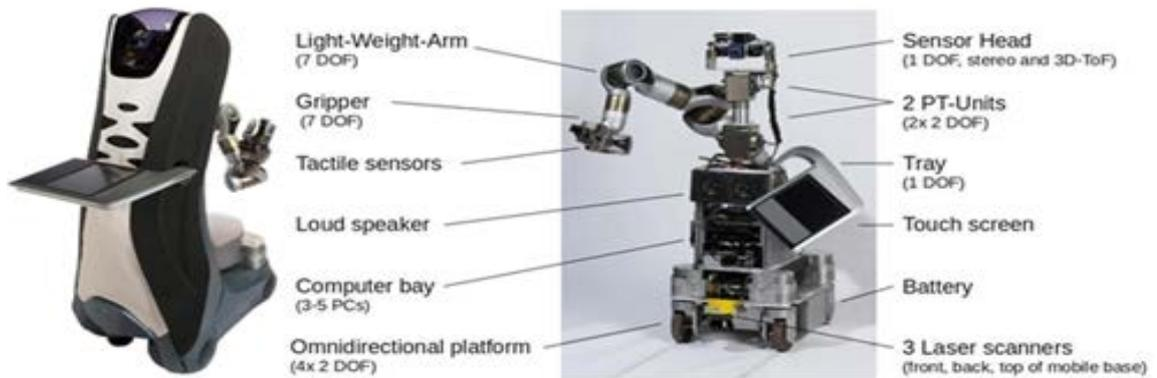
Figure 1-2: Care-O-Bot<sub>3</sub> platform (image courtesy of IPA, Fraunhofer)
