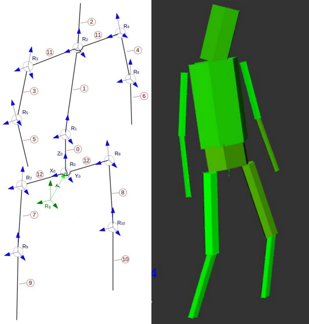
Figure 5-1: The simplified models used by the human pose estimation subsystem – left side, the articulated human body model; right side, the appearance model
