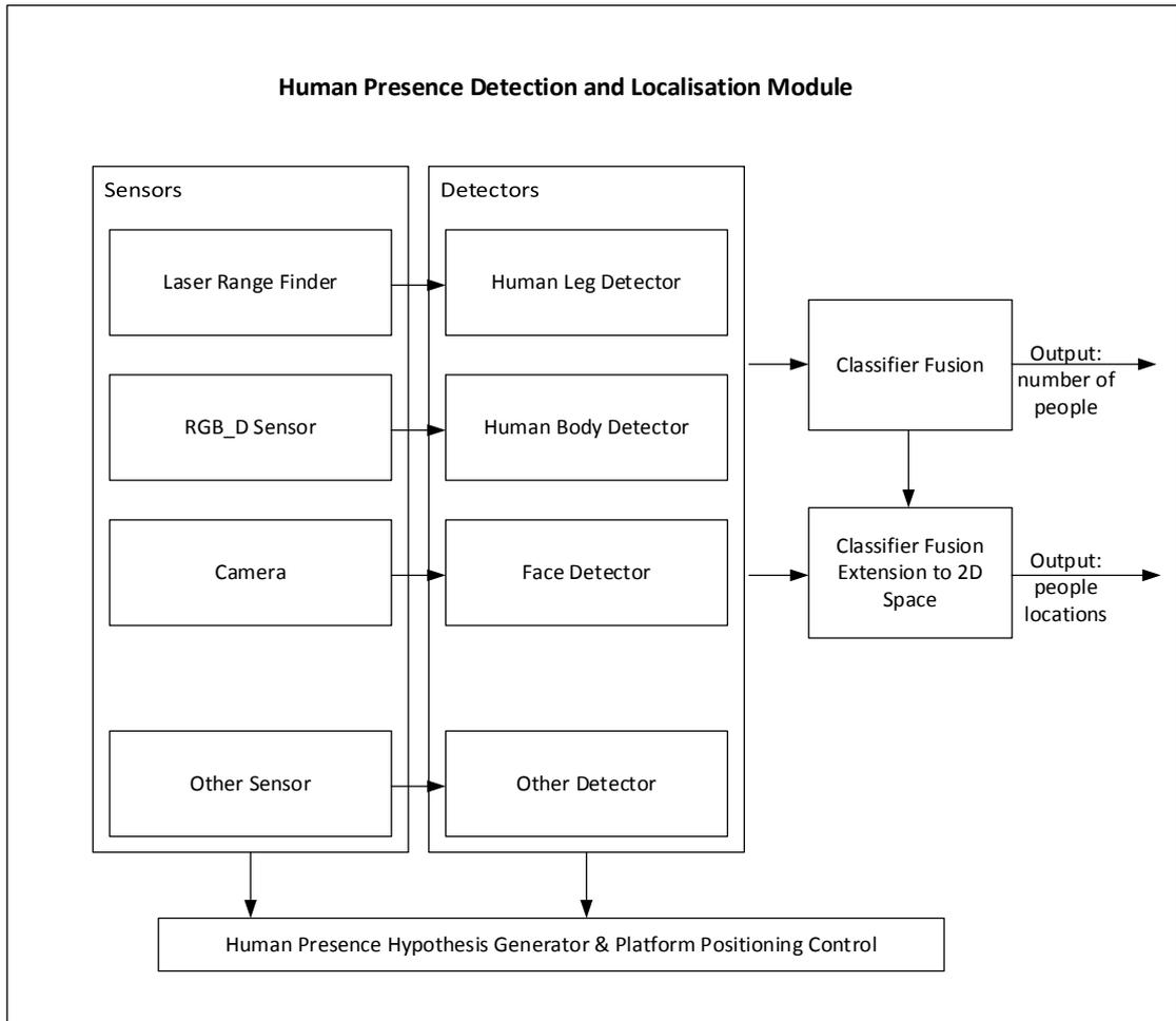
Figure 4-1: The conceptual model of the Human Presence and Localisation Subsystem
