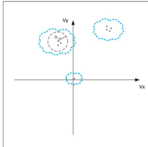
Figure 6-12: Clustering of the state of velocity components of tracks to form groups of people within each cluster of tracks
