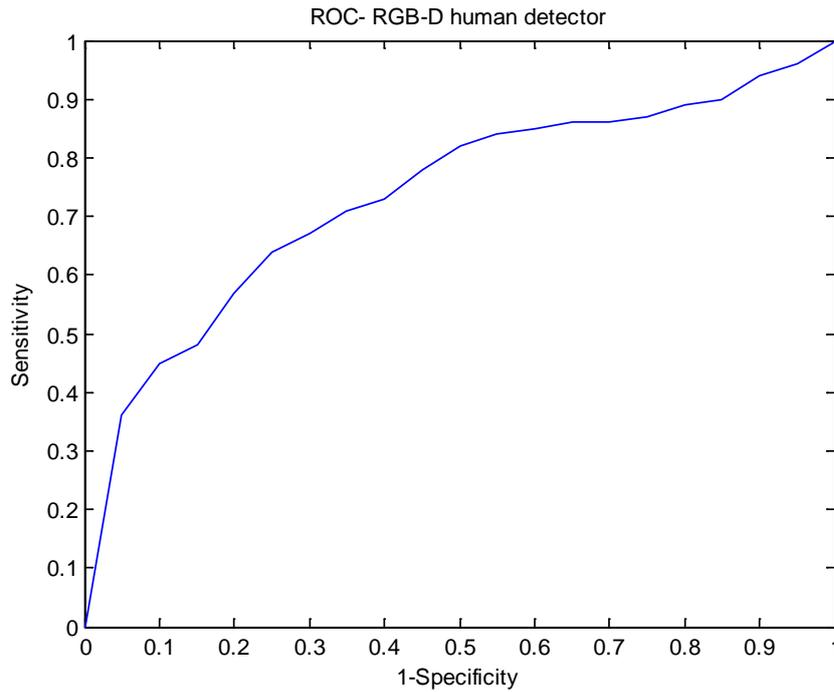
Figure 4-27: ROC curve of the RGB-D human detector
