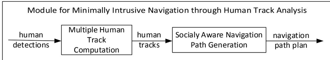
Figure 6-1: Conceptual overview of the Minimally Intrusive Navigation Subsystem
