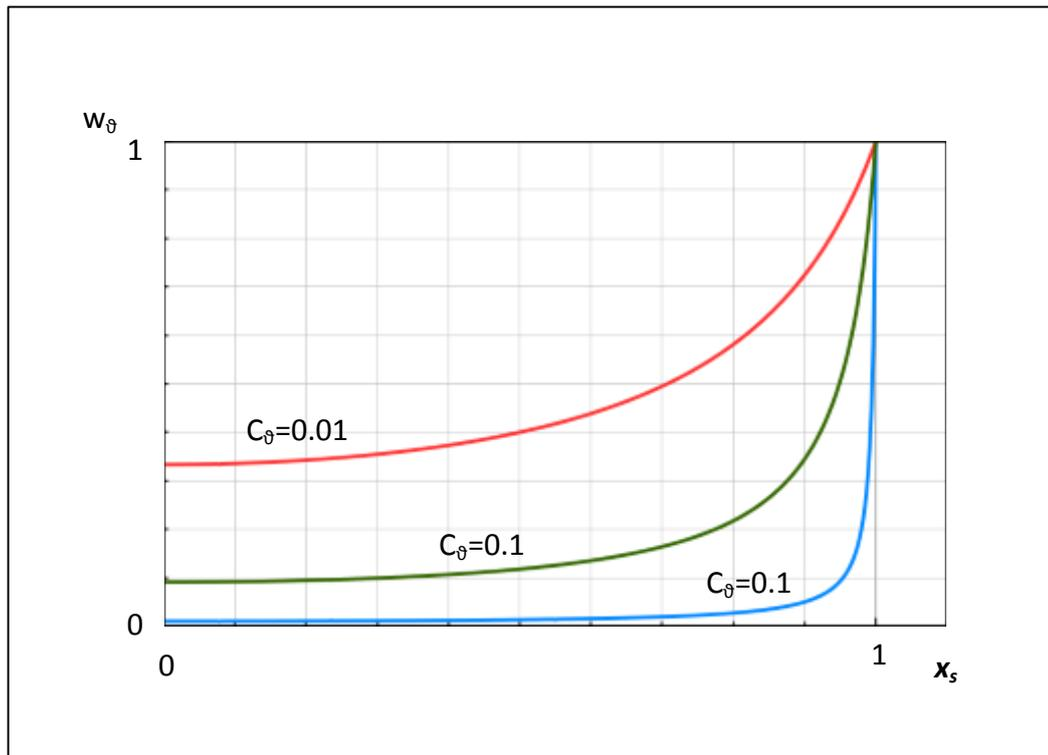
Figure 5-5: The weight function of the global optimisation part.
