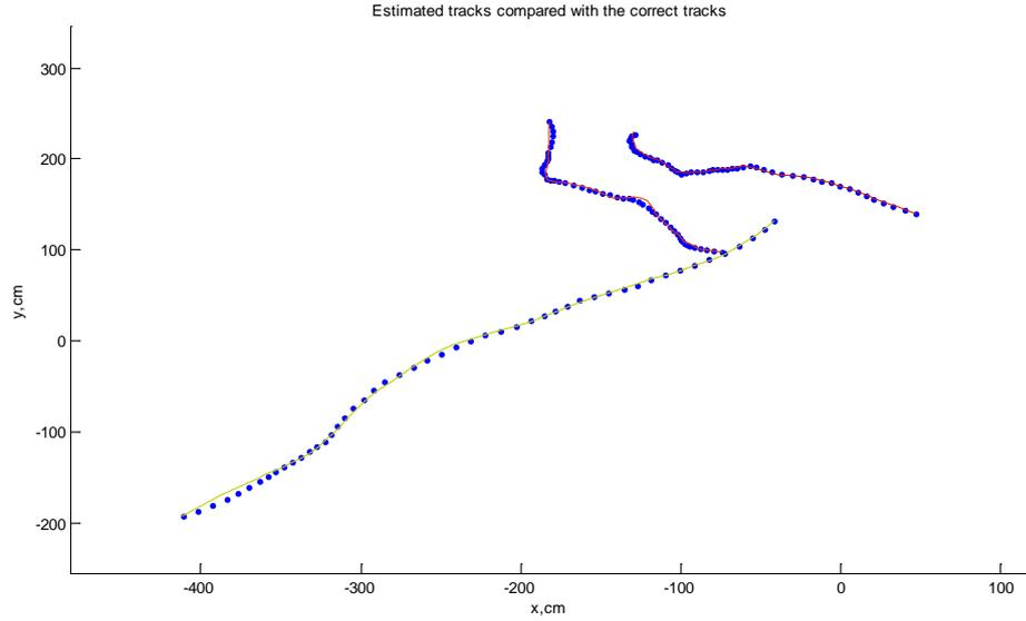
Figure 6-20: Estimated tracks in comparison with the correct tracks
