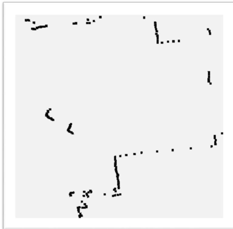
**Figure 4-2: A typical scan image from a laser range finder from a service robot in a home environment.** *Note: the chevrons in the middle represent detections of human legs*
