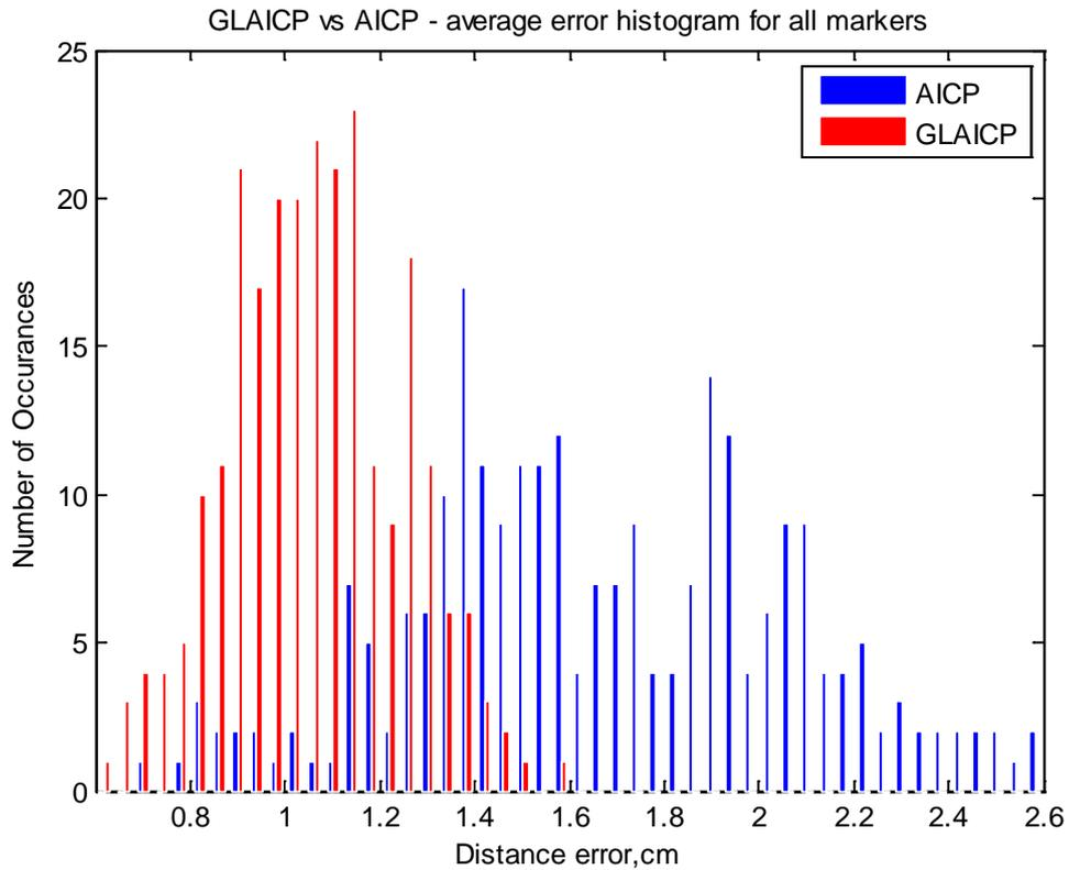
Figure 5-12: Distance error distributions of GLAICP and AICP algorithms
