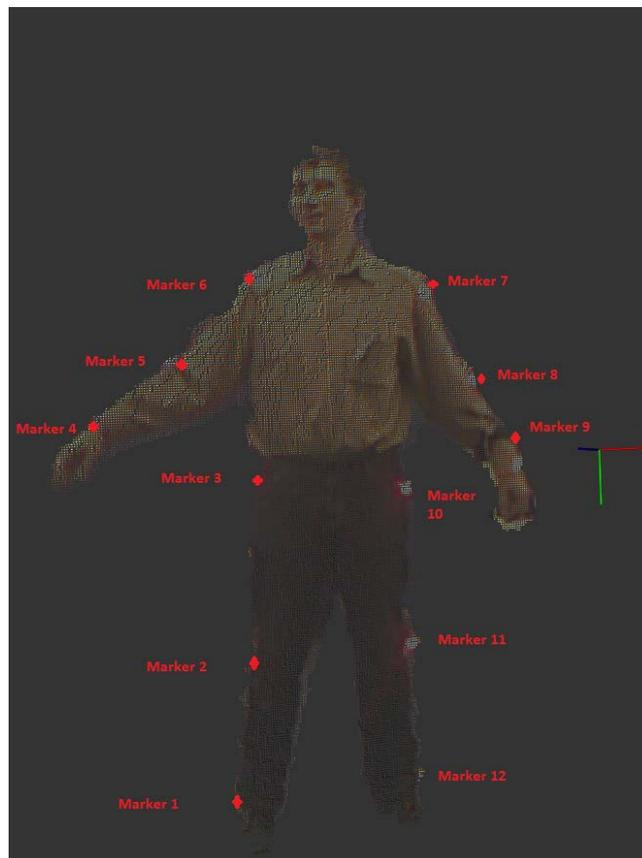
Figure 5-10: Position of the markers in the experimental setup (point cloud visualisation)
