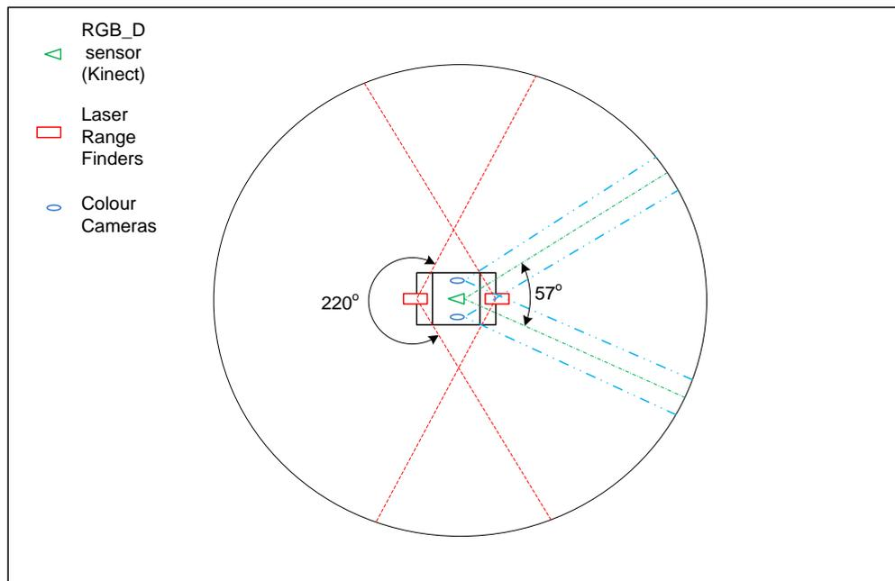
Figure 3-2: Experimental sensor spatial configuration - horizontal field of view
