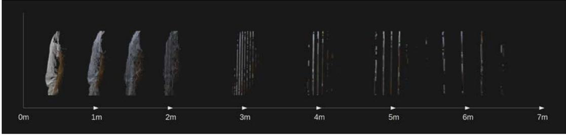
Figure 4-9: Effect of progressive loss of depth resolution of the Kinect sensor at different distances.
