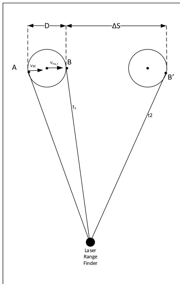
Figure 9-4: Calculation of the distortion resulting from the tangential leg motion component
