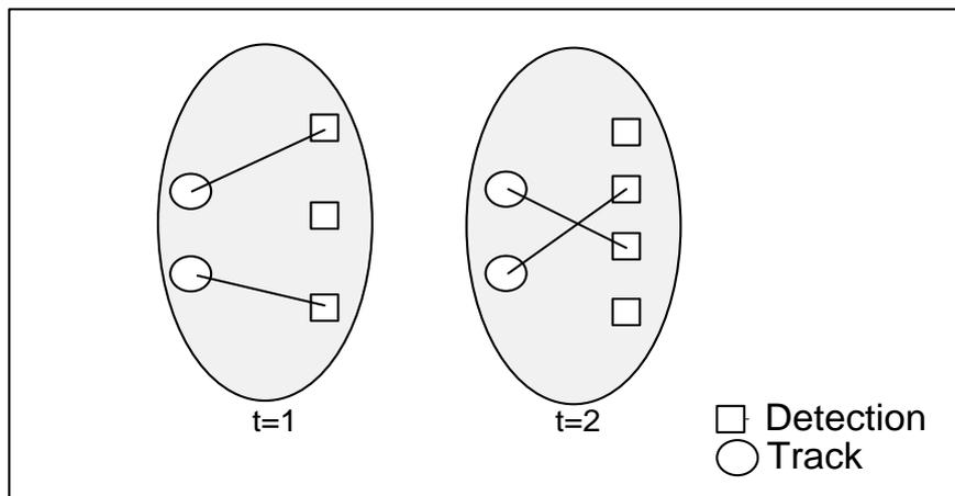
Figure 6-3: Illustrative example of data associations between two tracks and detections
