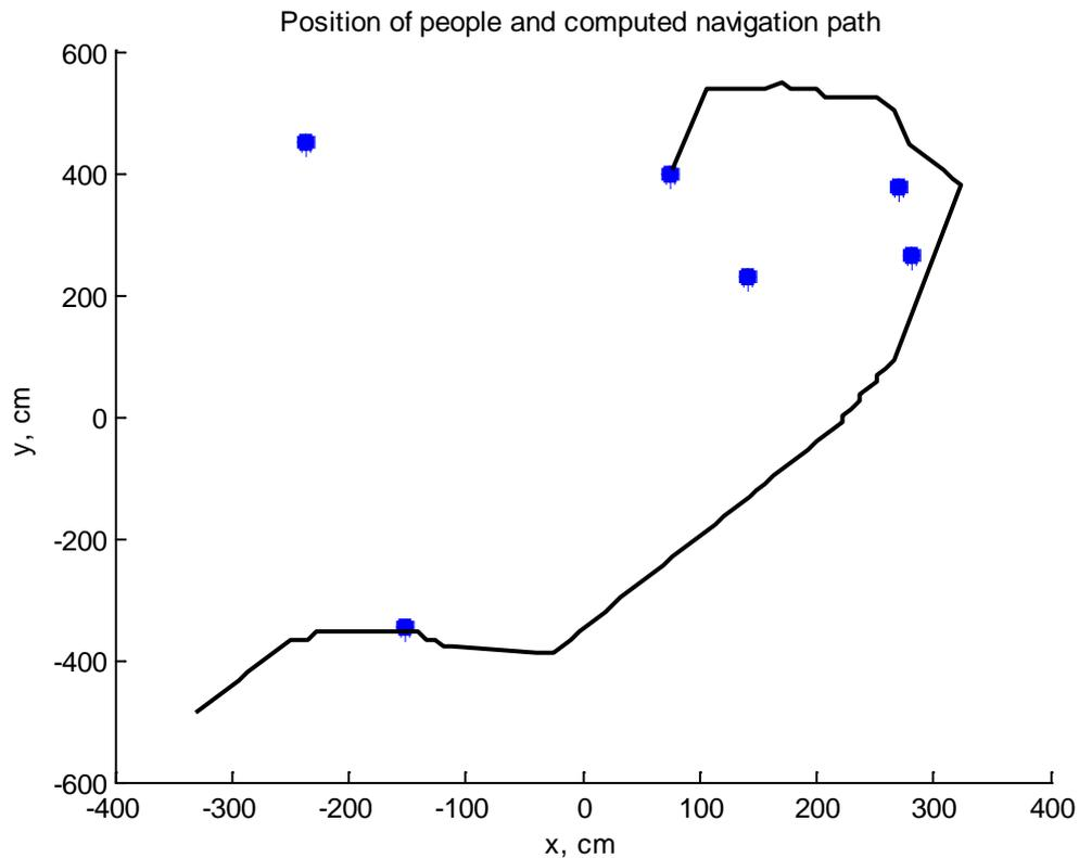
Figure 6-23: A typical navigation path computed by the algorithm
