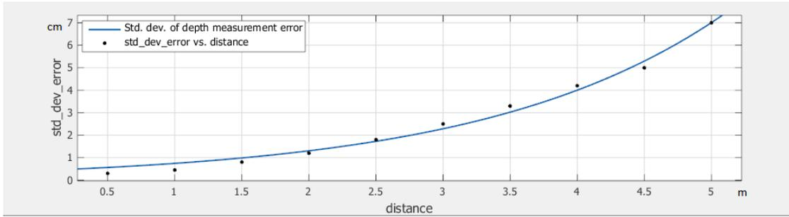
Figure 4-7: Model of the standard deviation of the Kinect's depth error
