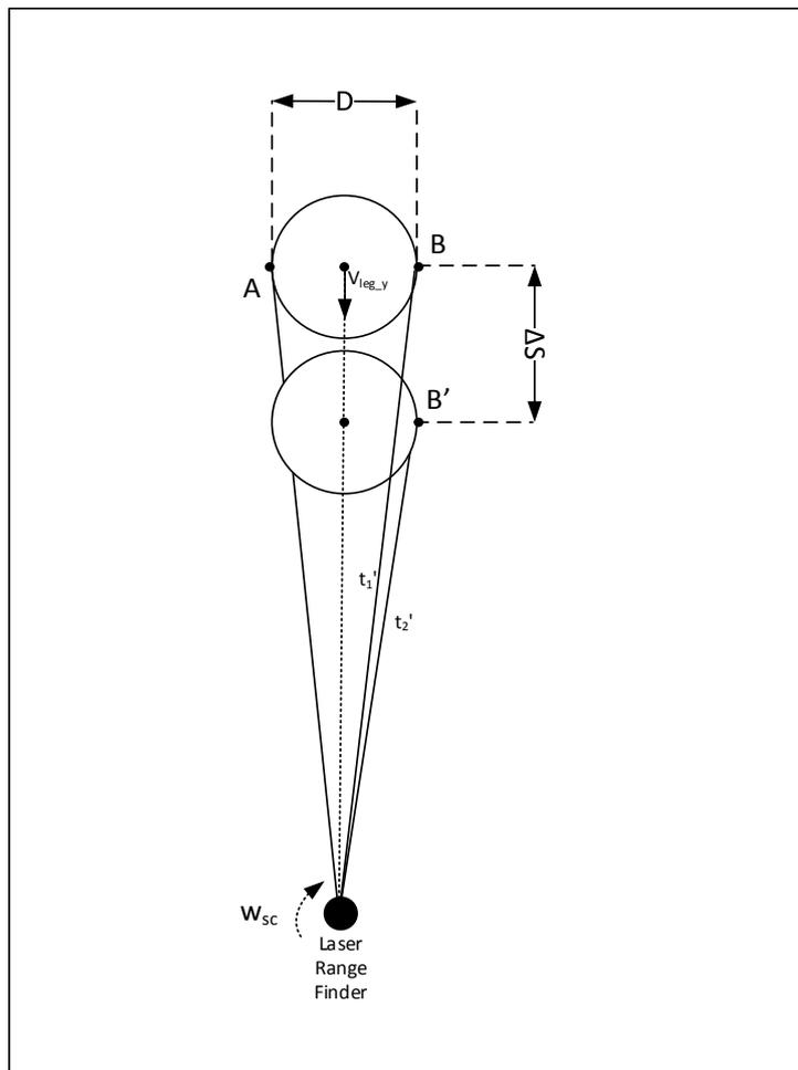
Figure 9-5: Computation of the distortion resulting from the radial leg motion component
