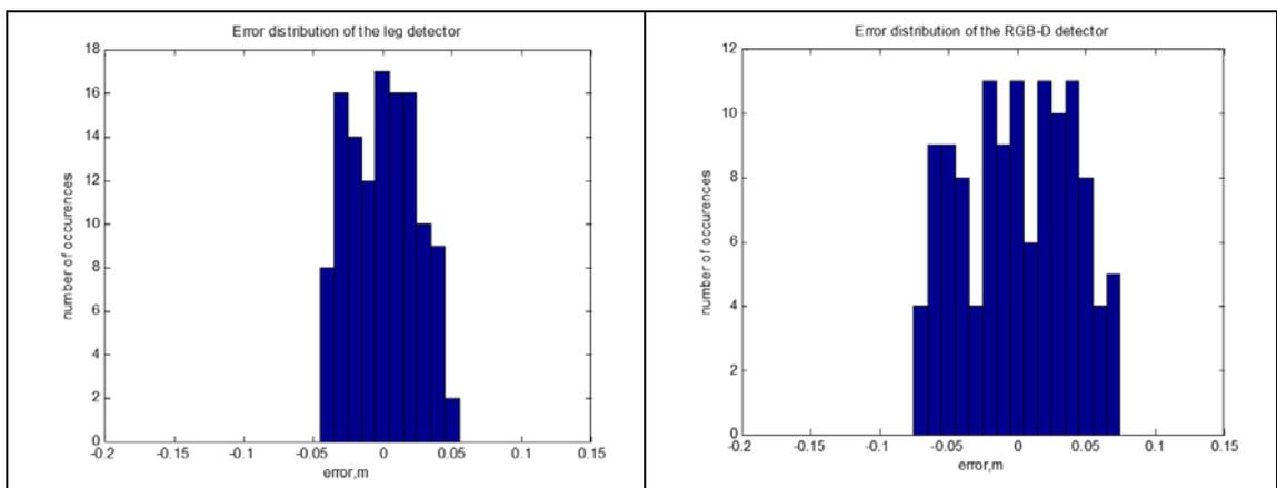
Figure 4-31: Comparison between distribution of the error of the leg and RGB-D detectors
