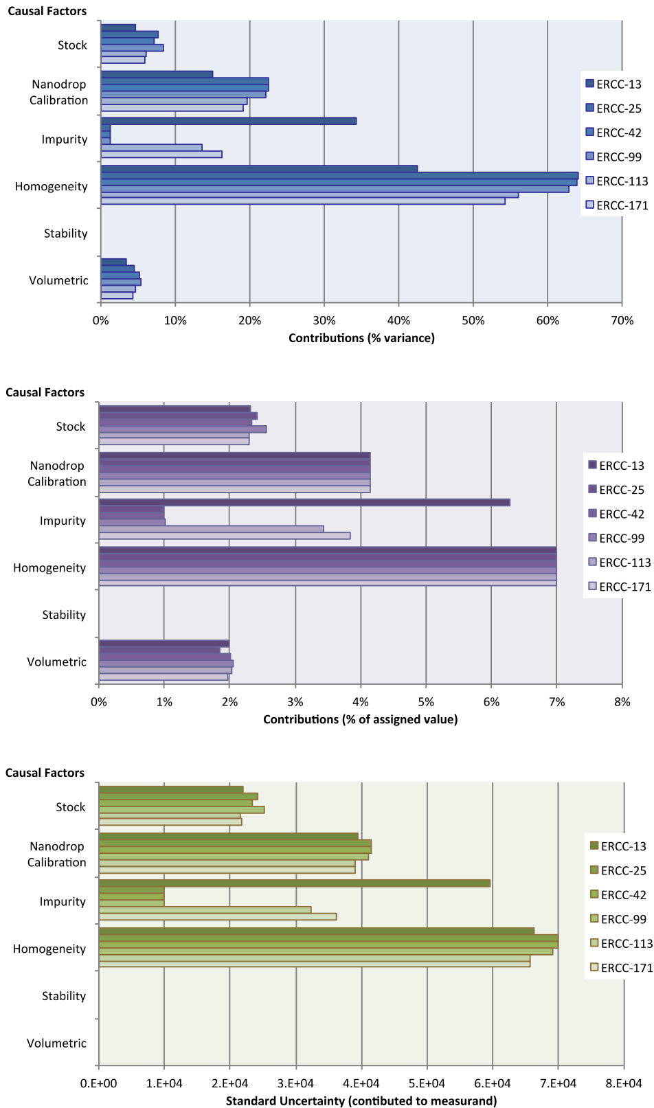
Figure 9.2 Calibrant Unit Measurement Uncertainty Contributing Factors. Purity assessment based on multiple banding (Bioanalyzer).
