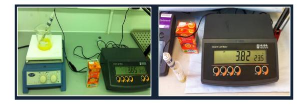
Figure 55. Measuring pH at room and body temperatures.
