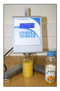
Figure 66. The rotational viscometer with a sample to test.
