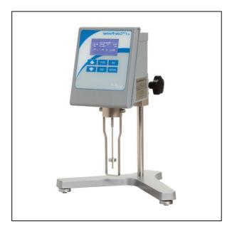
Figure 63. The basic rotational voscometer used in this part of study.
