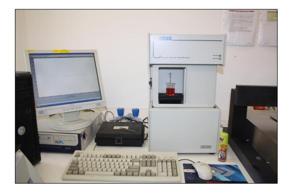
Figure 61. The dynamic contact angle analyser.
