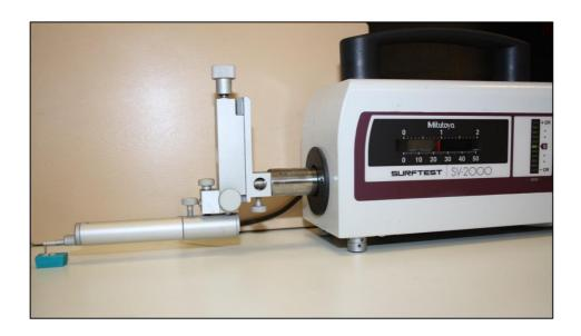
Figure 50. Three baseline readings using a contact surfometer were
