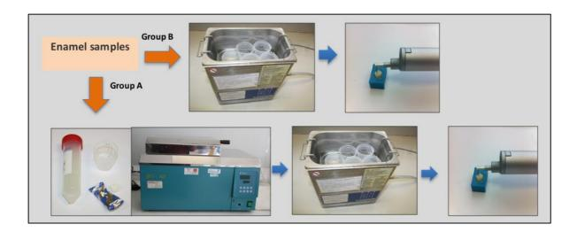
Figure 82. Subsuraface erosion test. Group A: immersing enamel samples in saliva for 1 hour then ultrasonication for 30 seconds then measured by surfometer, Group B: Immediate ultrasonication for 30 seconds then measured by surfometer.
