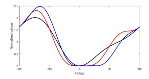
Fig. 9. Normalized voltage Third harmonic loads (a) and fundamental clipping contours (b) for 3 different cases, fixing  $Z_2 = (1 + j)R_{opt}/2$ .  $Z_3 = 0$  (black),  $Z_3 = 5R_{opt}$  (red), and  $Z_3 = (5 + j5)R_{opt}/\sqrt{2}$  (blue).
