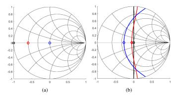
Fig. 3. Second harmonic loads (a) and fundamental clipping contour (b) for 3 different cases.  $Z_2 = 0$  (black square),  $Z_2 = R_{opt}/4$  (red diamond), and  $Z_2 = R_{opt}$  (blue circle).
