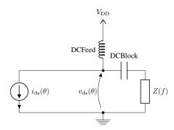
Fig. 1. Simplified schematic used for the analysis.
