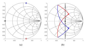
Fig. 2. Second harmonic loads (a) and fundamental clipping contour (b) for class B (black square), class J (red circle), and class  $J^{-1}$  (blue diamond).
