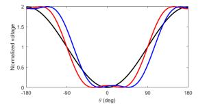
Fig. 7. Normalized voltage waveform for 3 different cases, fixing  $Z_2 = 0$ .  $Z_3 = 0$  (black),  $Z_3 = 5R_{opt}$  (red), and  $Z_3 = (5+j5)R_{opt}/\sqrt{2}$  (blue).
