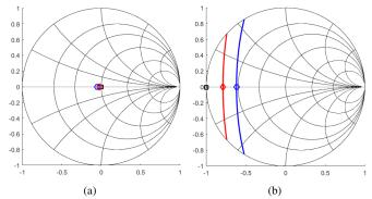
Fig. 5. Fundamental loads (a) and second harmonic clipping contour (b) for 3 different cases. Class B (black square),  $Z_1 = 0.95R_{\rm opt}$  (red diamond), and  $Z_1 = 0.9R_{\rm opt}$  (blue circle).
