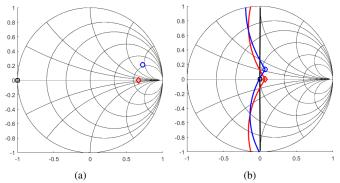
Fig. 6. Third harmonic loads (a) and fundamental clipping contours (b) for 3 different cases, fixing  $Z_2 = 0$ .  $Z_3 = 0$  (black square),  $Z_3 = 5R_{\rm opt}$  (red diamond), and  $Z_3 = (5 + j5)R_{\rm opt}$  (blue circle).
