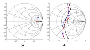
Fig. 8. Third harmonic loads (a) and fundamental clipping contours (b) for 3 different cases, fixing  $Z_2 = (1 - j)R_{\rm opt}/2$ .  $Z_3 = 0$  (black square),  $Z_3 = 5R_{\rm opt}$  (red diamond), and  $Z_3 = (5 + j5)R_{\rm opt}/\sqrt{2}$  (blue circle).
