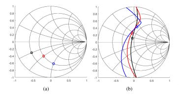
Fig. 4. Second harmonic loads (a) and fundamental clipping contour (b) for 3 different cases.  $Z_2 = (1-j)R_{opt}/4$  (black square),  $Z_2 = (1-j)R_{opt}/2$  (red diamond), and  $Z_2 = (1-j2)R_{opt}/2$  (blue circle).
