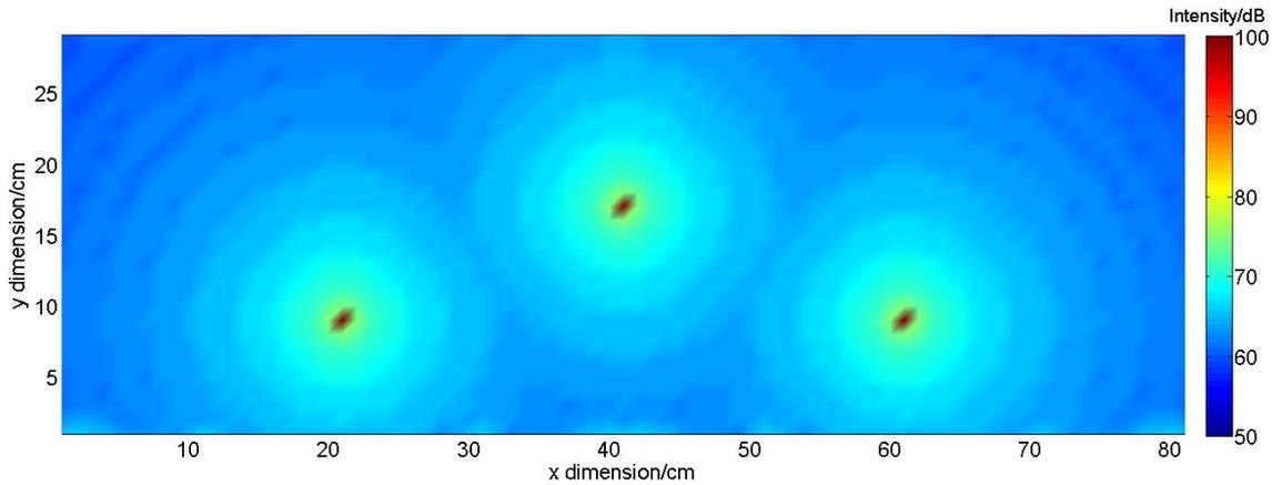
**Figure 2. Intensity plot for a three-sensor network**
