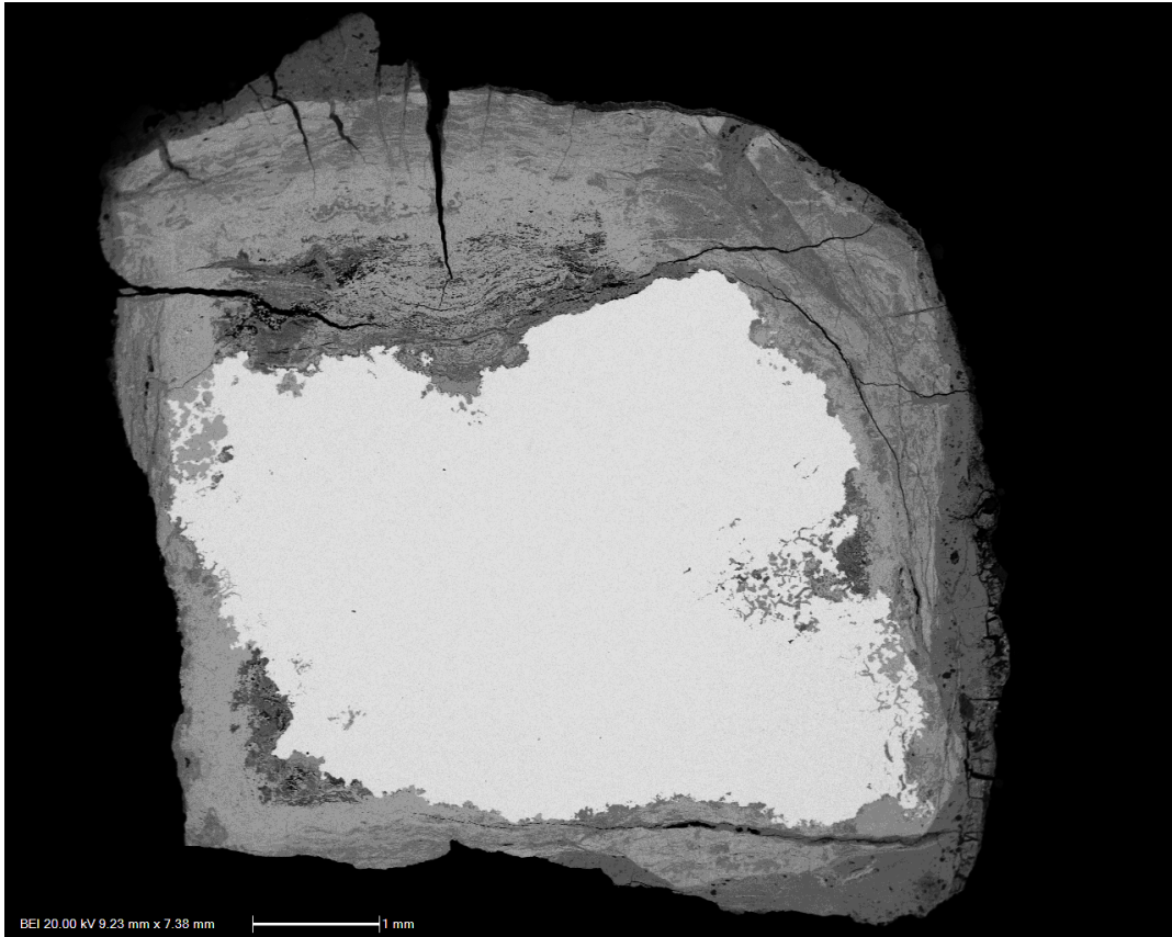
Figure 5.6 SEM-BSE image of Caerleon nail CAER_13 post alkaline sulphite treatment in polished cross-section at 13X magnification showing metal core, corrosion pits, thick DPL of up to 2615 \mu\text{m} , TM and extensive concentric and radial cracking. Scale bar=1mm
