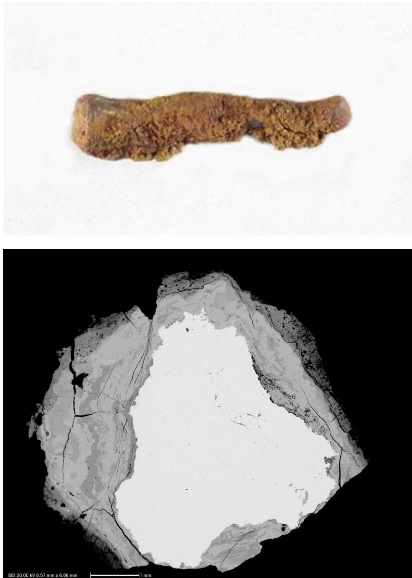
Figure 4.1 Digital photograph at 1.5X (top) and SEM-BSE image at 20X (bottom) of nail sample CAER_01 from Caerleon
