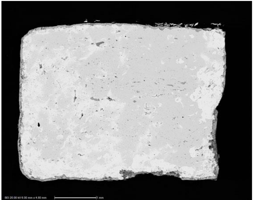
Figure 8.15 SEM-BSE image of Colonial Williamsburg nail CW_14 in polished cross-section at 20X magnification.
