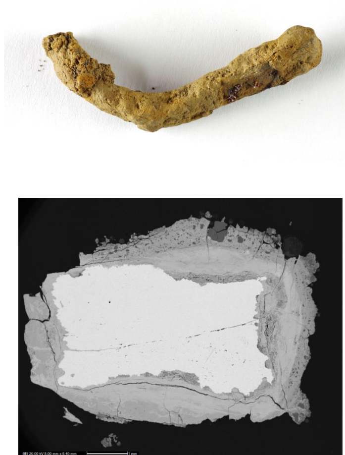
Figure 5.1 Digital photo at 1:1 scale (top) and SEM-BEI cross-sectional image (bottom) of CAER_10 a wrought iron nail from Caerleon. Voluminous corrosion product layers of varying thickness and degrees of cracking can be seen. Scale bar=1mm.
