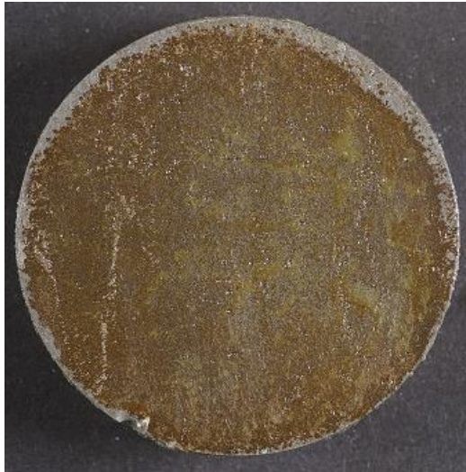
Figure 212 PB72PC1B – top side cleaned, corroded and coated
