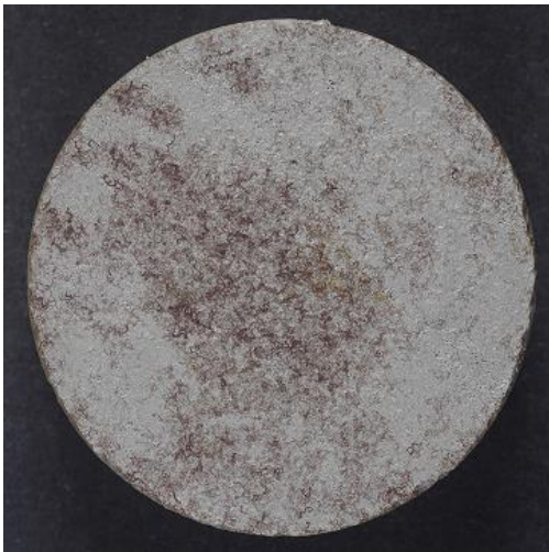
Figure 182 PC1A after exposure at 80% RH for 48 days
