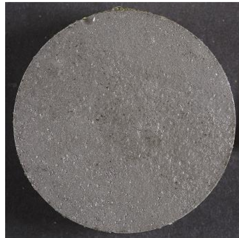
Figure 189 PB72CS5B after coating with 3 layers of 10% w/v Paraloid B72 in acetone before O 2 monitoring
