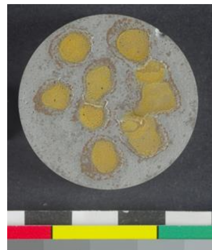
Figure 108 Sample corroded by salt solution applied by pipette
