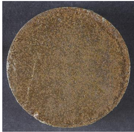
Figure 213 PB72PC1B after exposure at 80% RH for 342 days
