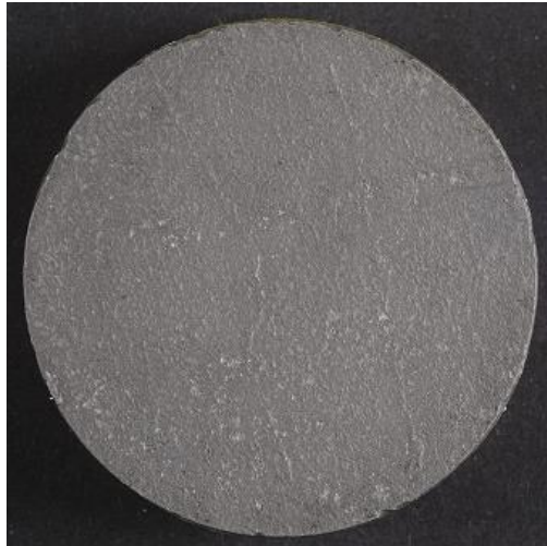
Figure 196 CH80CS5A after coating with 3 layers of 10% w/v Cosmoloid H80 in white spirit before O 2 monitoring
