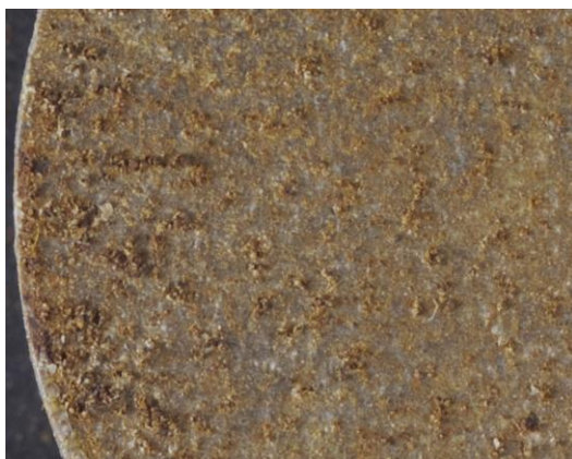
Figure 219 Zoomed area of CH80PC2B with loose corrosion and small fragments of detaching coating
