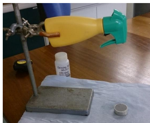
Figure 90 Spray bottle/sample set up.
