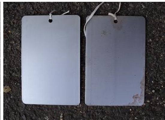
Figure 65 Front and back of two of the plates that were placed in position on the 1st October 2013 and were assessed on 19 th May 2014. The plate from inside the bag (left-hand side of both images) suffered no corrosion, but the one in the area surrounding the tank has significant areas of corrosion (Delaney, 2015).
