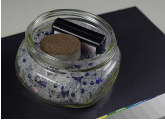
Figure 91 Jar setup - pink O 2 sensor spot adhered inside the jar, conditioned silica gel, data logger and sample.
