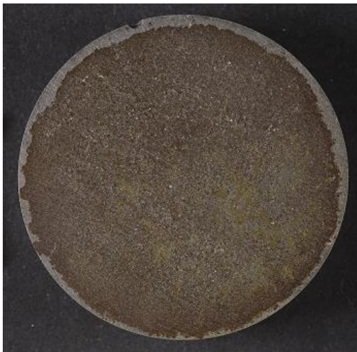
Figure 222 S10PC6B – coating applied over the corrosion caused by sprayed salt solution
