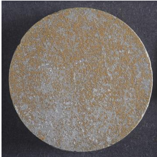
Figure 198 CH80CS5A after monitoring O 2 levels for 341 days
