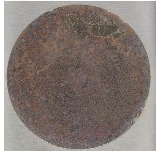
Figure 165 UT1B after 163 days exposed to 80% RH
