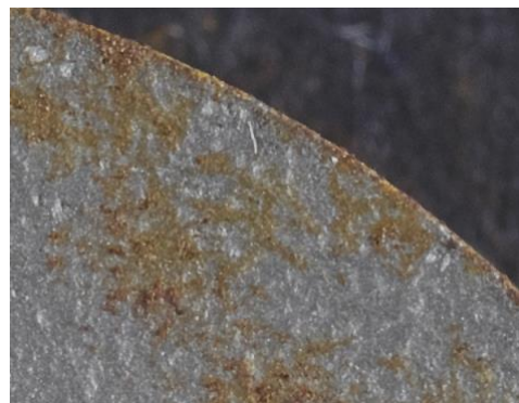
Figure 209 Zoomed area of corrosion on sample S10CS5B
