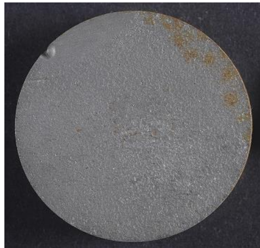
Figure 207 S10CS5B after monitoring O 2 levels for 341 days
