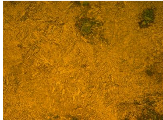
X50 Magnification - Etched weld area
