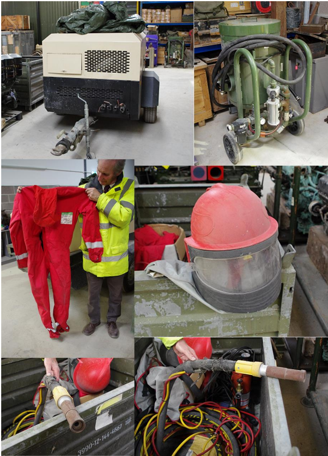
Figure 68 Machinery and safety equipment used by the Tank Museum for grit blasting armoured vehicles in preparation for painting (displayed by Mike Hayton, workshop manager at the TM).
