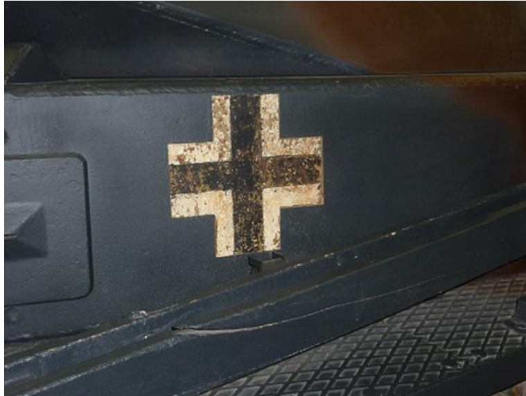
Figure 70 A cleaned and painted armoured vehicle on display at the Tank Museum with historic paint detail left intact, but requiring additional protection, ideally a clear coating.
