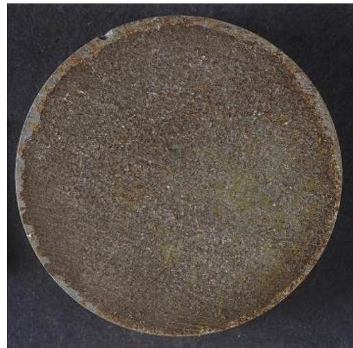
Figure 223 S10PC6B after exposure at 80% RH for 342 days
