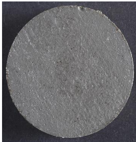
Figure 191 PB72CS5B after O 2 monitoring for 341 days – minimal corrosion visible
