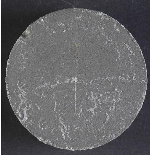
Figure 225 PB72 coated, scribed sample 1 side B with salt solution painted down the scribe in the coating to accelerate corrosion
