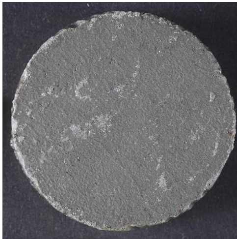
Figure 190 PB72CS5A after O 2 monitoring for 341 days – minimal corrosion visible
