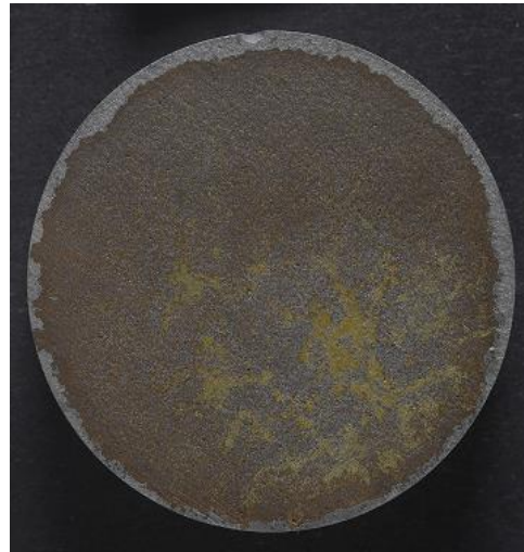
Figure 221 S10PC6B – top side sprayed with salt solution, after corroding for 8 days
