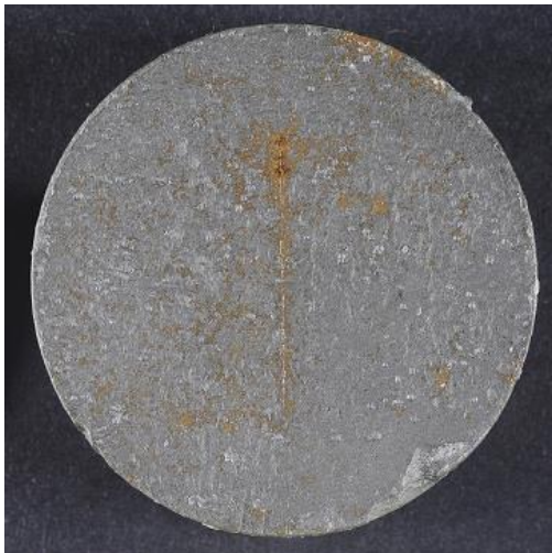
Figure 231 CH80SC5A after monitoring O 2 levels for a further 148 days – 218 days in total
