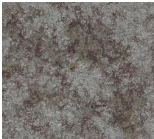
Figure 244 Zoomed central area of sample PC5 after exposure at 80% RH
