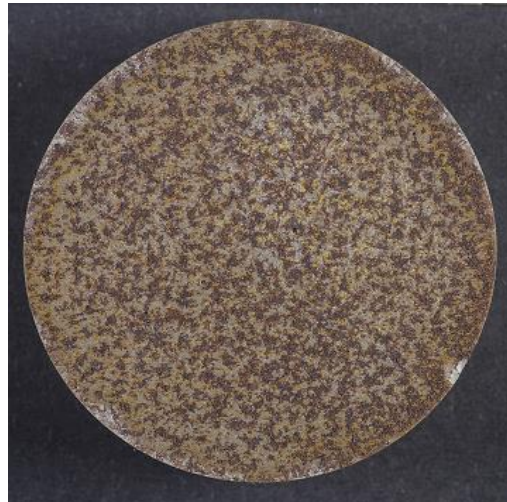
Figure 183 PC1B change in corrosion after exposure at 80% RH for 48 days
