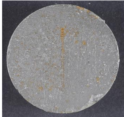
Figure 230 CH80SC5A after monitoring O 2 levels for 70 days, showing yellow-brown general corrosion
