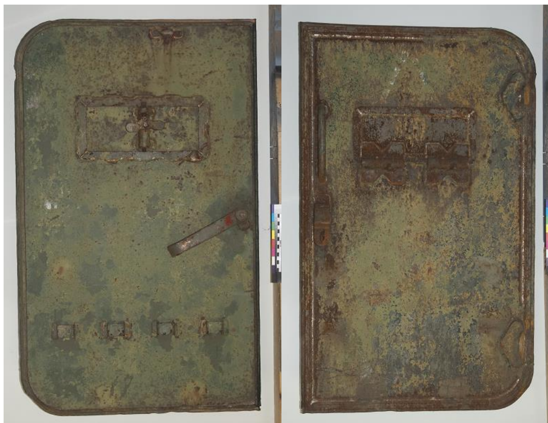
Figure 87 Both sides of the Saracen APV door – laid flat and photographed from above
