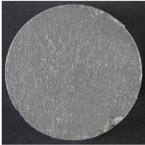
Figure 229 CH80 coated, scribed sample 5 side A with salt solution painted down the scribe in the coating to accelerate corrosion
