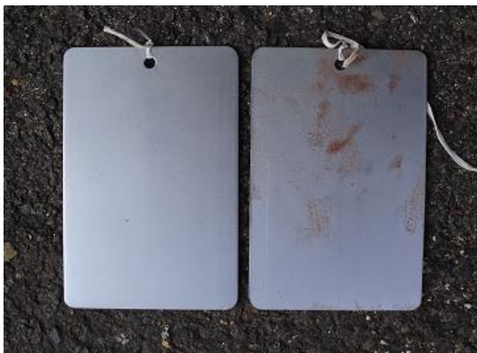
Figure 65 Front and back of two of the plates that were placed in position on the 1st October 2013 and were assessed on 19 th May 2014. The plate from inside the bag (left-hand side of both images) suffered no corrosion, but the one in the area surrounding the tank has significant areas of corrosion (Delaney, 2015).
