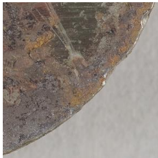
Figure 167 Zoomed area of UT1B after 163 days exposed to 80% RH
