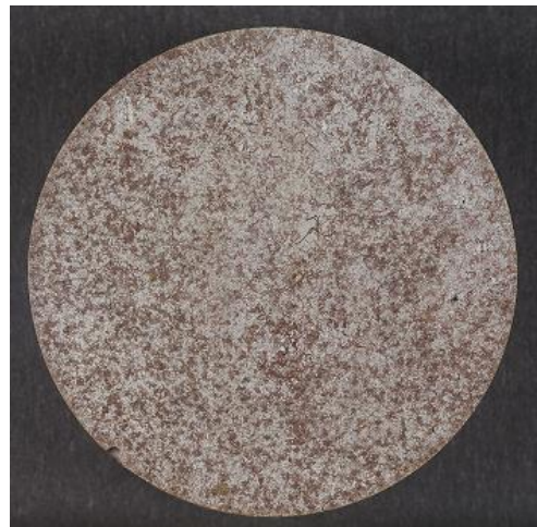
Figure 173 CS3B after exposure at 80% RH for 65 days
