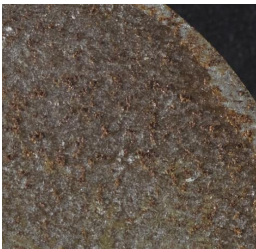
Figure 224 Zoomed area of S10PC6B revealing powdery corrosion
