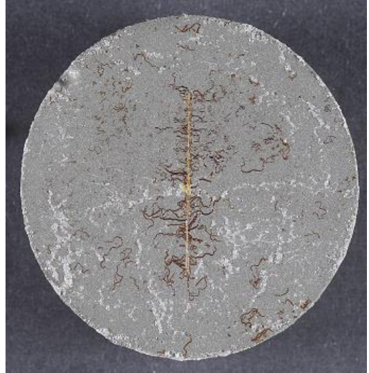
Figure 226 PB72SC1B after monitoring O 2 levels for 70 days, clearly showing filiform corrosion
