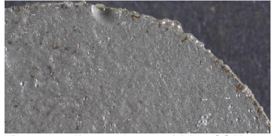
Figure 193 Zoomed area of PB72CS5B highlighting corrosion patches and bubbles within the coating.
