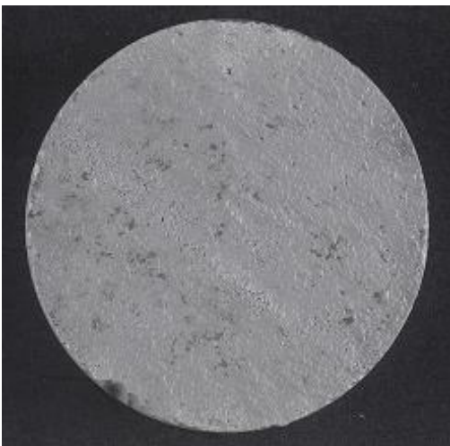
Figure 170 CS3A after air abrading before exposure at 80% RH
