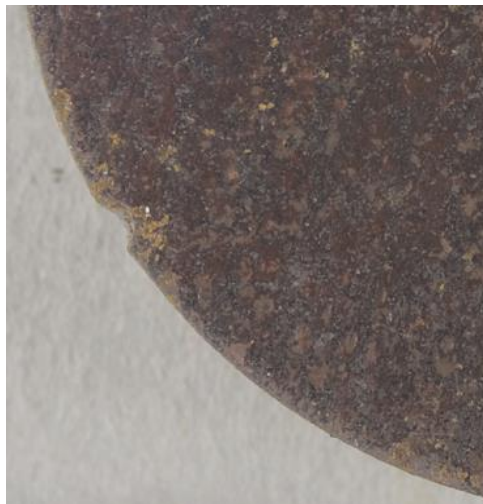
Figure 166 Zoomed area of UT1A after 163 days exposed to 80% RH
