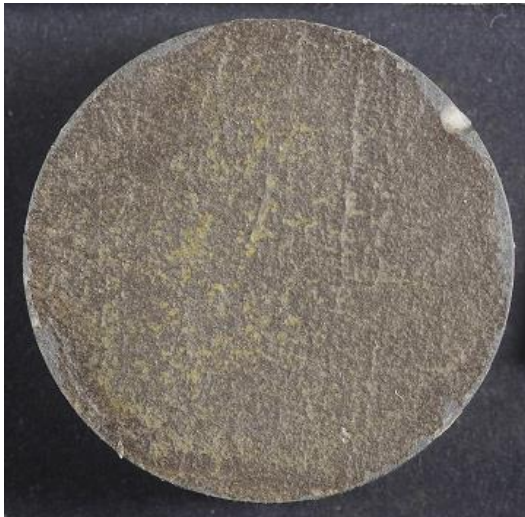
Figure 217 CH80PC2B – top side cleaned, accelerated corroded and then coated
