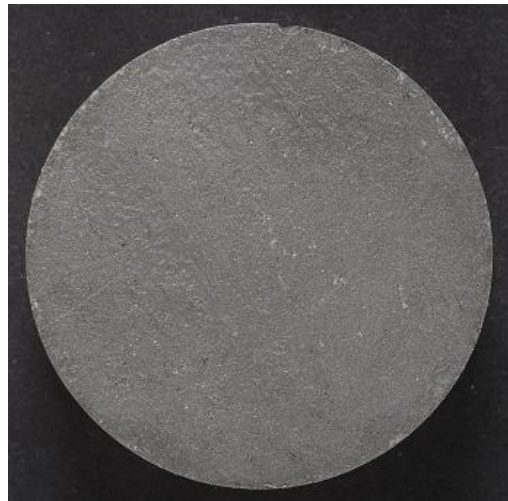
Figure 197 CH80CS5B after coating with 3 layers of 10% w/v Cosmoloid H80 in white spirit before O 2 monitoring
