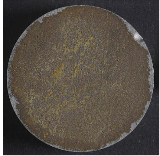
Figure 216 CH80PC2B – top side sprayed with salt solution and allowed to corrode for 8 days
