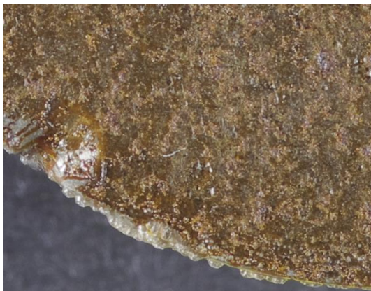
Figure 214 Zoomed area of PB72PC1B - filiform corrosion at the edge and bubbles in the coating.
