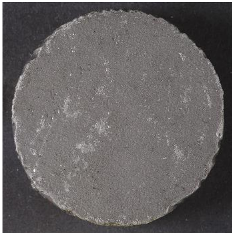
Figure 188 PB72CS5A after coating with 3 layers of 10% w/v Paraloid B72 in acetone before O 2 monitoring
