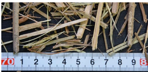
Figure 4. 5A first stage of cutting and grinding of a whole frond of Iraqi date palm (8mm as received)
