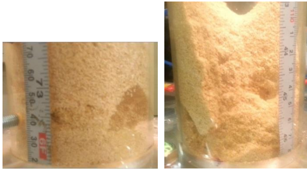
Figure 6. 3 Images of fluidisation behavior for air- SPWB system for air flowrates from 0.0 to 120 l/min.
