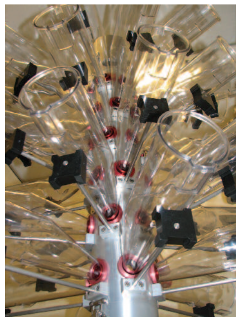
Snout-only inhalation exposure chamber with rat restraint tubes
