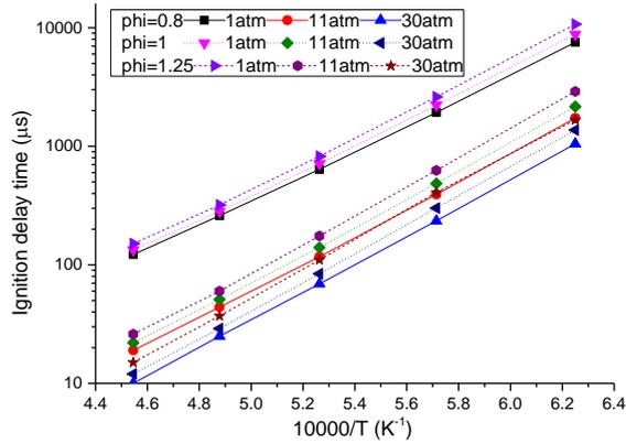
Fig. 4. Ignition delay time of ammonia/methane mixture
