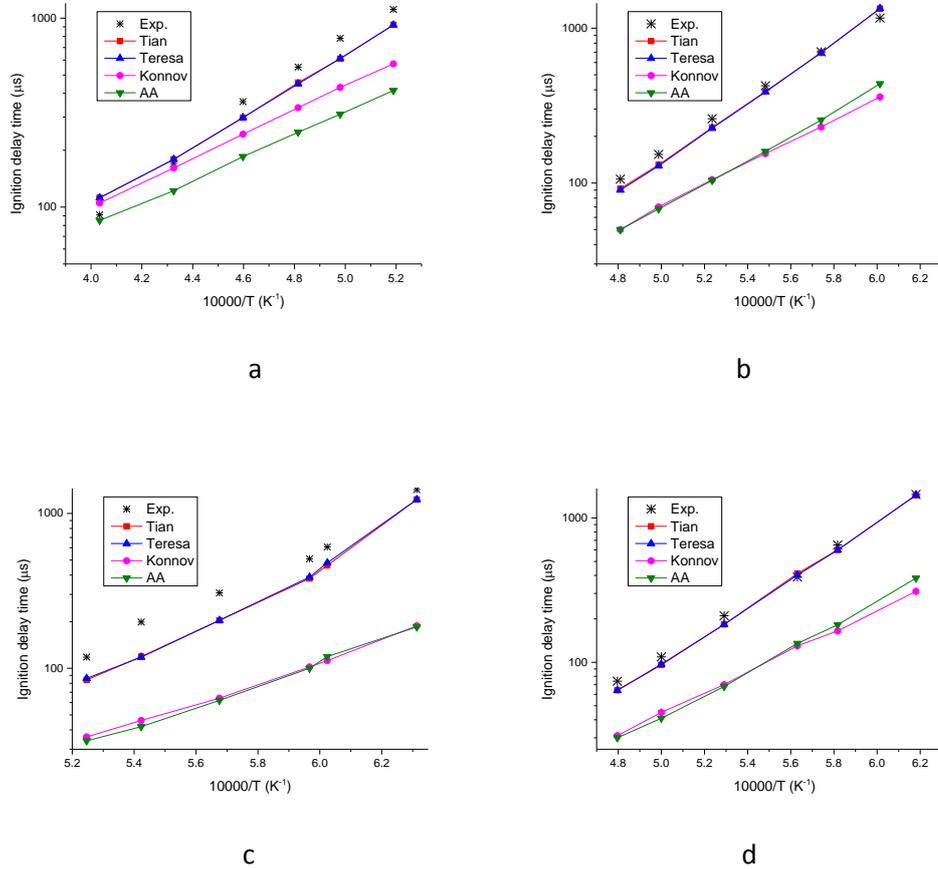
**Fig. 3.** Performance of different mechanisms with respect to ignition delay times of  $\text{NH}_3$  mixtures. a) 1.4 atm, E.R. = 0.5, 99% Ar; b) 11.0 atm, E.R. = 1.0, 99% Ar; c) 30.0 atm, E.R. = 2.0, 99% Ar; d) 11.0 atm, E.R. = 1.0, 98% Ar. Experiments as in [14].
