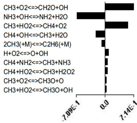
**Fig. 8.** OH sensitivity using Tian mechanism.
