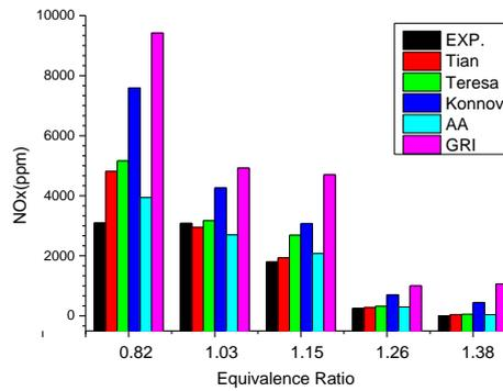
Fig. 5. NO<sub>x</sub> emission under STP condition. Experiments as in [29].
