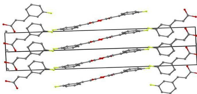
**Figure 3.7.** Crystal structure of the  $\beta_2$  polymorph of 3-FCA viewed along the  $[110]$  direction, showing the two orientations of the molecular planes. Only the orientation of the fluorophenyl rings corresponding to the major disorder component, is shown in the packing diagram. For clarity, hydrogen atoms are omitted from the structure.
