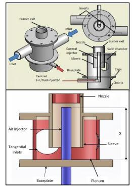
Figure 1. 150 kW tangential swirl burner
