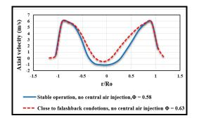
Figure 6. Change in axial velocity when equivalence ratio increased from stable to flash back conditions (no central air injection).
