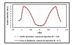
Figure 7. Change in axial velocity when equivalence ratio increased from stable to flash back conditions (with central air injection).
