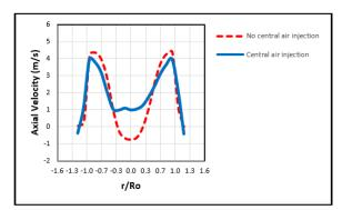
Figure 2. LDA results, effect of air injection on axial velocity downstream burner mouth (Y/D=0.0816)
