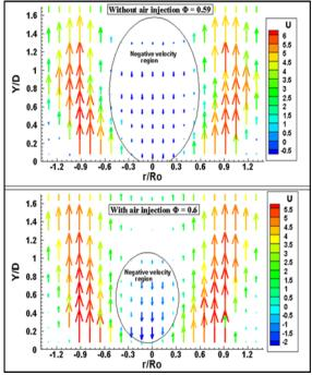
Figure 3. LDA results, effect of air injection on axial velocity magnitude downstream burner mouth at different distances (Y/D)
