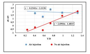
Figure 5. LDA results, variation of axial velocity gradient downstream burner mouth
