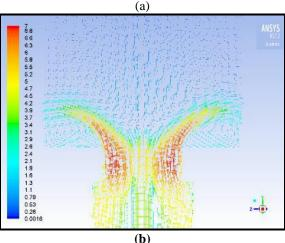
Figure 4. CFD results, (a) without air injection (b) with air injection, diffusive air injection pushes the CRZ downstream, consequently, prevent CIVB.
