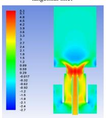
Figure 4. Axial velocity contour (m/s), 600 LPM tangential inlet, X=150 mm
