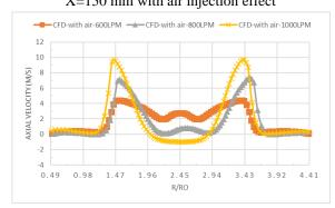
Figure 6. Axial velocity comparison for different tangential inlets at P2, X=150 mm
