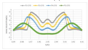
**Figure 5**. Axial velocity at different planes form burner mouth, 600 LPM tangential inlet, X=150 mm with air injection effect
