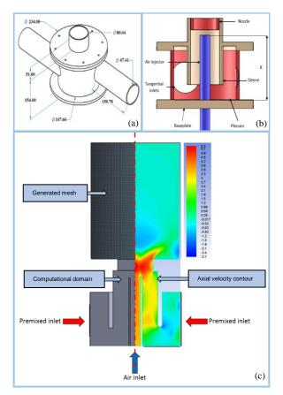
**Figure 1**: Schematic view of the computational domain, Physical model, mesh, and axial velocity contour (600 LPM with air injection)
