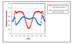
**Figure 7**. CFD results, three-dimensional turbulent intensity values, effect of central air injection, 600 LPM, at P2 plane, X=150 mm
