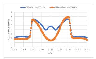
Figure 3. Effect of axial air injection on the defect of axial velocity at P2 with X = 150 mm, 600 LPM tangential inlet
