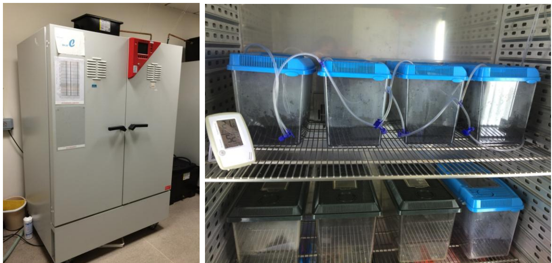
Figure 5.3: Environmentally-controlled cabinet used to keep rearing containers for caddisfly pupae under laboratory conditions.
