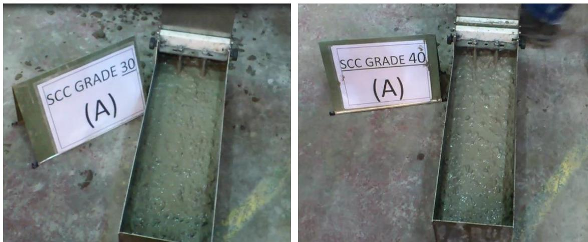
Figure 5.13: Passing and filling of SCC mix: 30A (Left), 40A (Right)
