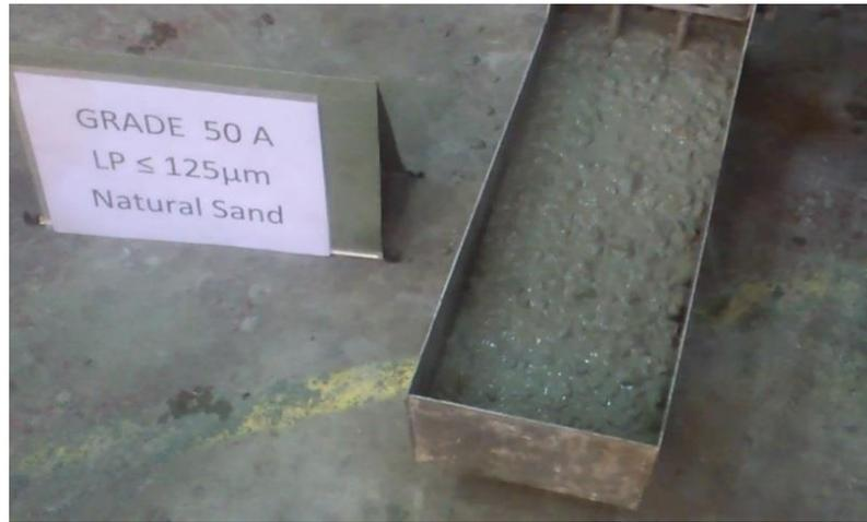
Figure 5.15: Passing and filling of SCC mix (50A)
