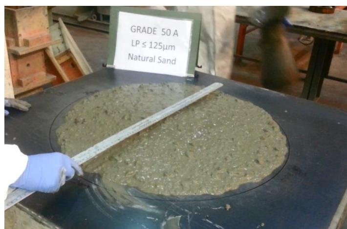
Figure 5.4: Horizontal spread of SCC mix (50A)
