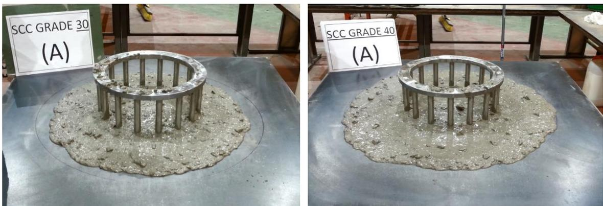
Figure 5.9: Flow and passing ability of SCC mix: 30A (Left), 40A (Right)
