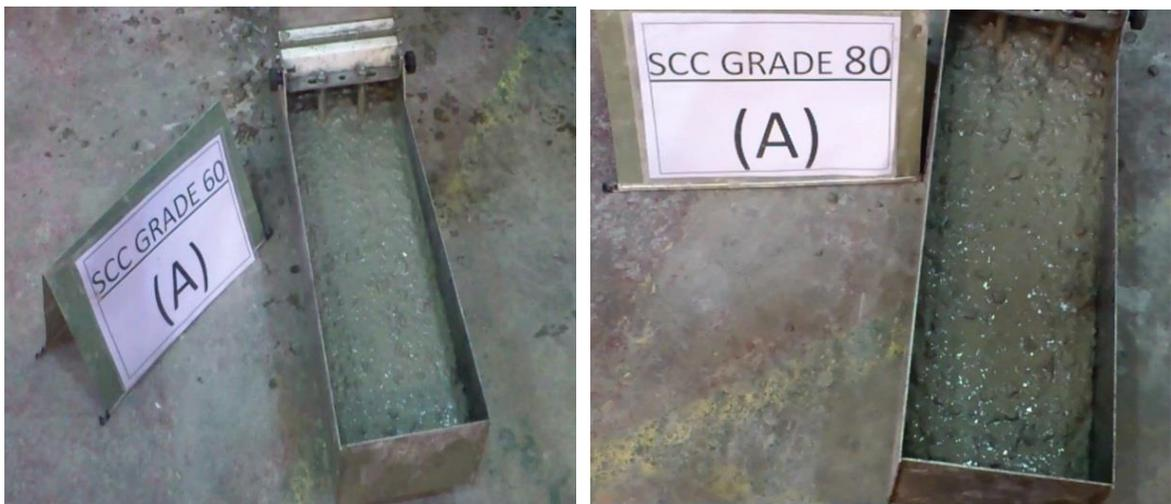
Figure 5.14: Passing and filling of SCC mix: 60A (Left), 80A (Right)
