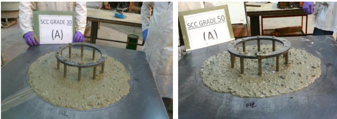
**Figure C.1: Flow and passing ability of SCC mix: 30A (Left), 50A (Right)**
