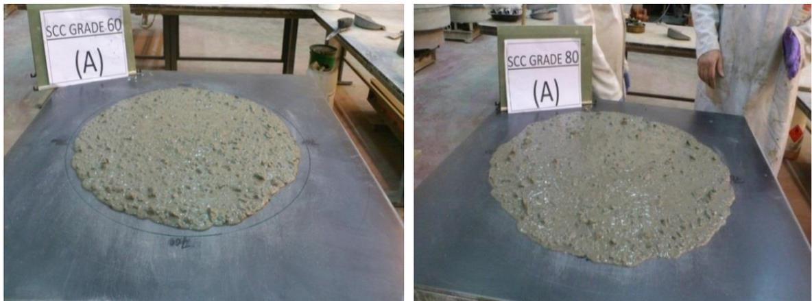
Figure 5.3: Horizontal spread of SCC mix: 60A (Left), 80A (Right)
