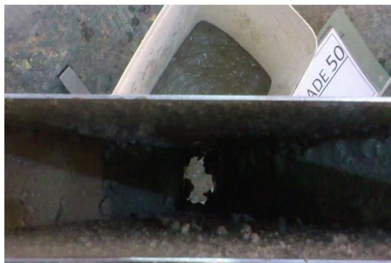
**Figure 5.1: Recording V-funnel time (daylight appearing when viewed from above)**
