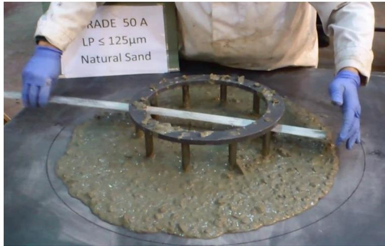
Figure C.3: Flow and passing ability of SCC mix (50A)
