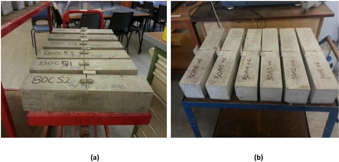
Figure 6.4: (a) shallow notch to depth ratio (0.1), (b) deep notch to depth ratio (0.6)
