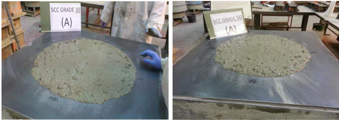
Figure 5.2: Horizontal spread of SCC mix: 30A (Left), 50A (Right)
