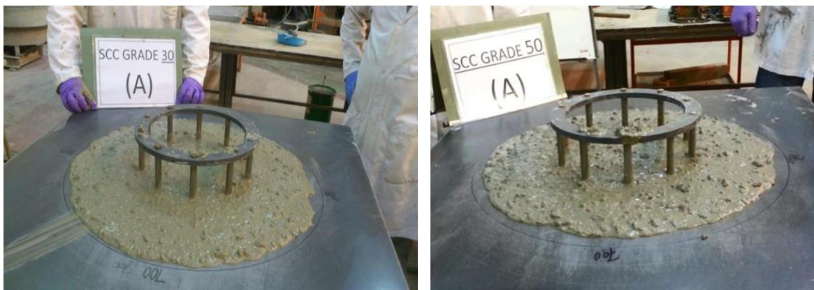
**Figure C.1: Flow and passing ability of SCC mix: 30A (Left), 50A (Right)**
