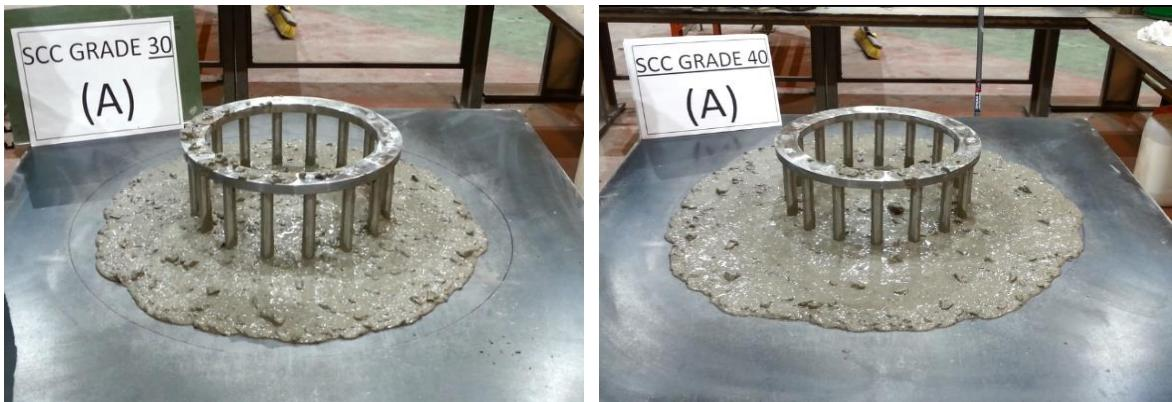
**Figure 5.9: Flow and passing ability of SCC mix: 30A (Left), 40A (Right)**
