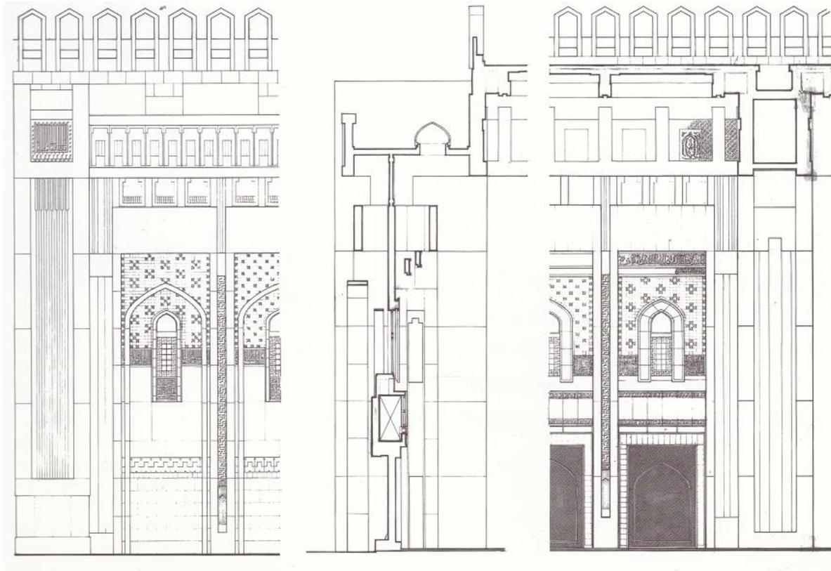
Figure 8.27: From left: exterior elevation of the wall bay unit, section of the wall bay unit and section-elevation of the interior wall bay units and decorations. Source: (Kanan, 1990, p. 67).
