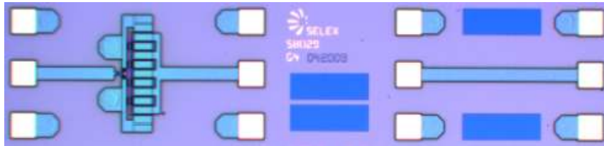
Figure 3.4 MMIC test cell photograph from RFMD FD30 mask 58029.0001.001 MM1465A showing a 10x75 \mu\text{m} transistor test cell and the RF ‘thru’ calibration structure.
