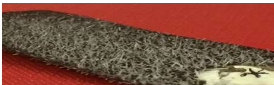
Figure 5.10 Precipitates covered cathode surface
