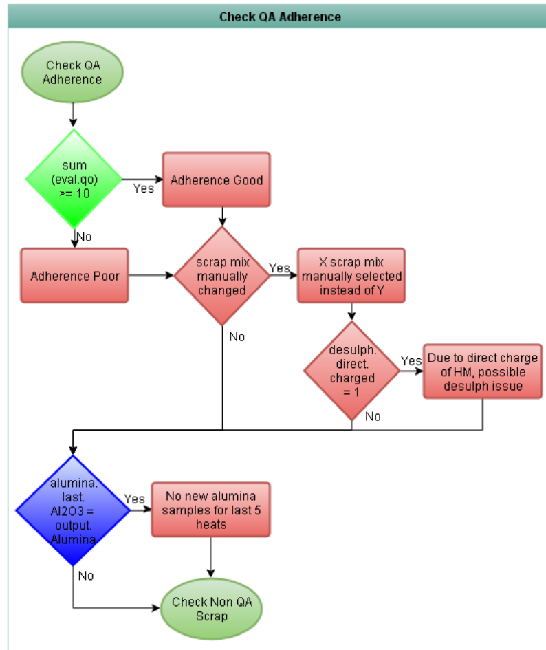
Figure 3.30 – Flow Diagram Showing Process Logic Used For QA Adherence Outputs
