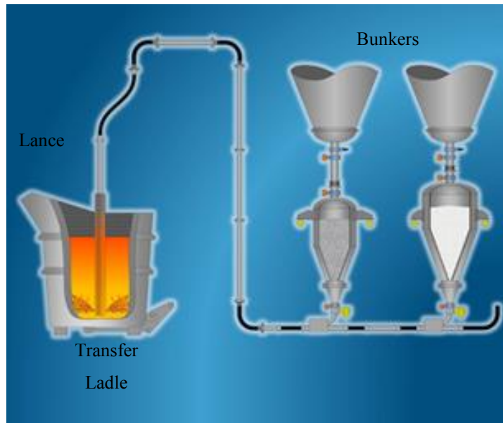
Figure 1.4 Basic Schematic Of Desulphurisation Process, Reproduced from (ThyssenKrupp, n.d.)
