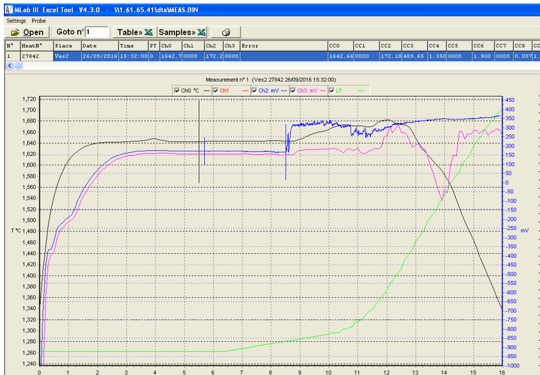
Figure 5.37 - Multilab Output For Quality Codes, The Codes Being Based On How Flat The Signal Is
