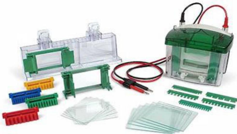
**Figure 2.6.4** The Mini-PROTEAN Tetra handcast system (Bio-Rad Laboratories, URL).
