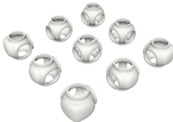
Figure 13. Rule definition of cellular units for corner, edge, and interior conditions.
