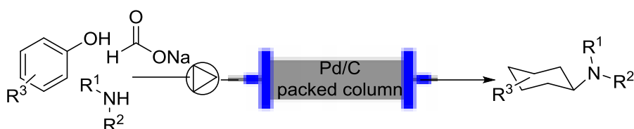
Figure 3.23: Synthesis of cyclohexylamines by reduction of phenol and subsequent reductive amination by Pd/C and sodium formate in a cartridge flow reactor.
