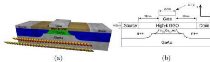
Figure 1: (a) 3D model of  $\text{In}_{0.3}\text{Ga}_{0.7}\text{As}$  MOSFET showing spin polarization of electrons along  $n$ -channel with 4% strain in the [001] direction (Red) and unstrained (Purple). (b) Schematic of  $\text{In}_{0.3}\text{Ga}_{0.7}\text{As}$  MOSFET.
