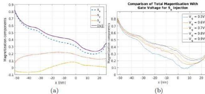
Figure 2: (a) Magnetisation components vs. position along the channel (averaged over 10 runs) taken for  $S_x$  injection at  $t = 8ps$ , i.e., after a steady state was reached. (b) Total magnetisation versus position at  $t = 8ps$  with different gate voltages ( $V_g$ ) and a fixed source-drain voltage ( $V_d$ ) of 0.9 V.
