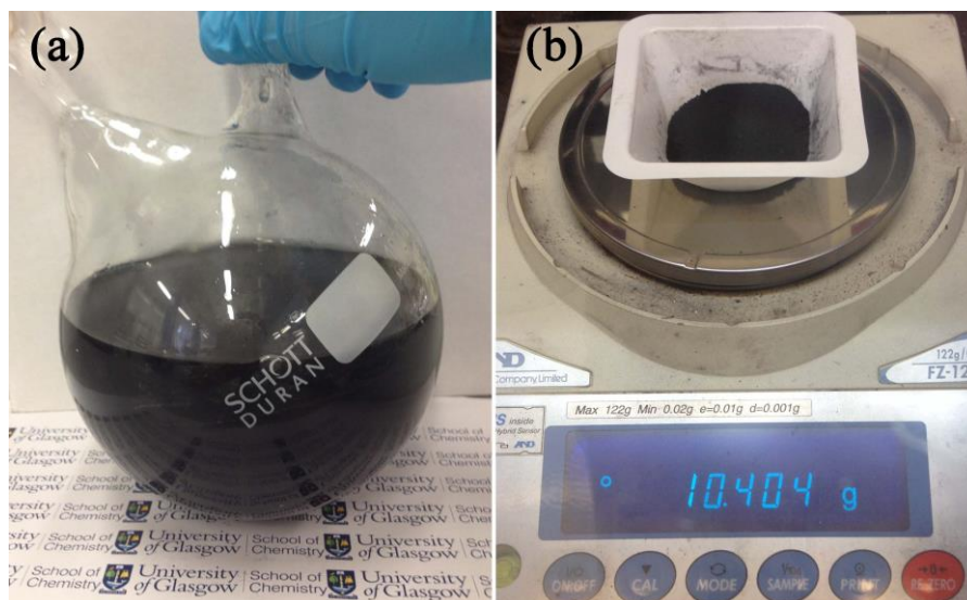
Figure S1. Digital photographs showing (a) the nanoparticle solution after a synthesis and (b) a typical yield of SnSe nanoparticles ( \sim 10.4 g, ca. 96 %) produced in a one-pot synthesis.
